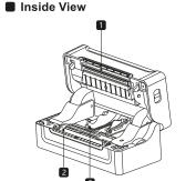
1.Thermal Head Piece 2.Rubber Roller 3.Paper Guide
