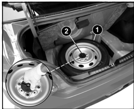
1. Spare Wheel 2. Retaining Bolt
