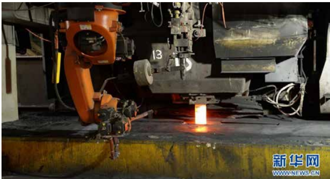
Exhibit 11: Remote Control of Robotic Arm for Slagging
