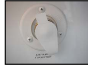
Figure 11-6. City Water Inlet
