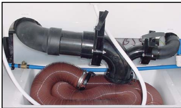
Figure 11-11. Sanitation Coupling, Valve, and Hose
