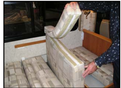
Figure 5-7. Filler Strip Attached to the Seat Portion
