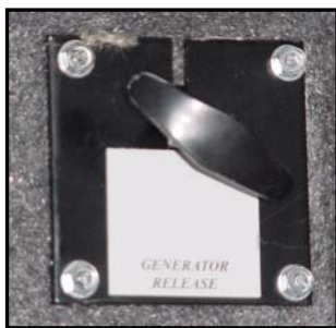
Figure 7-15. Generator "Pull" Cable Slide-Lock Release
