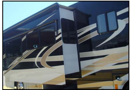
Figure 8-2. Typical Slide-Out Fully Extended
