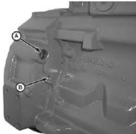
Flywheel Housing Timing Holes
