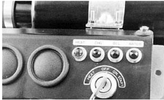
Key Switch in "ON" Position (4.5 L "270" Engines)
