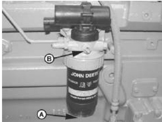
Drain Primary Fuel Filter (If Equipped)
