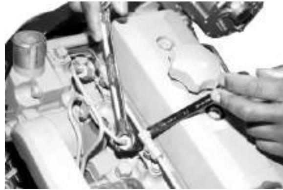
Bleed At Fuel Injection Nozzles
