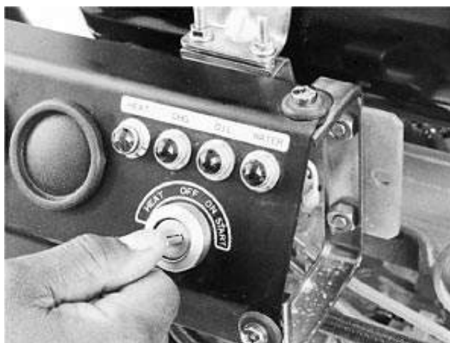
Starting Engine Using Key Switch (Earlier Engines)
