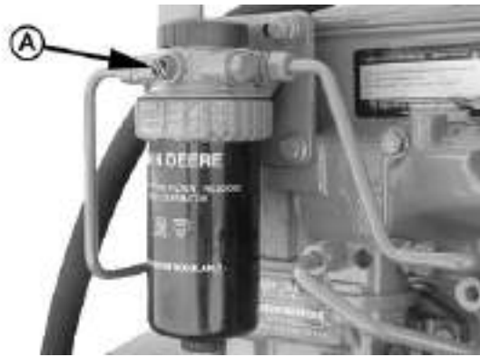
Final Fuel Filter Bleed Vent Screw
