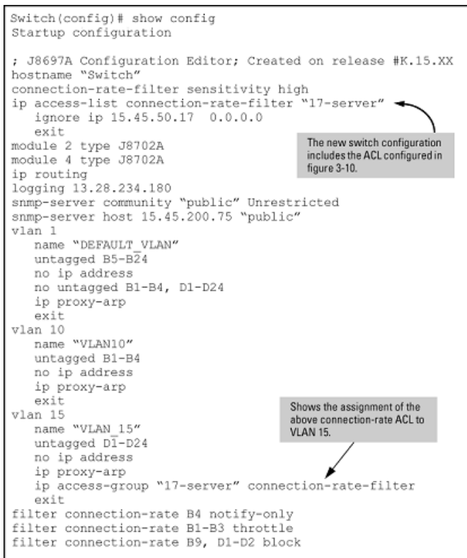
Figure 15 Example of switch configuration display with a connection-rate ACL
