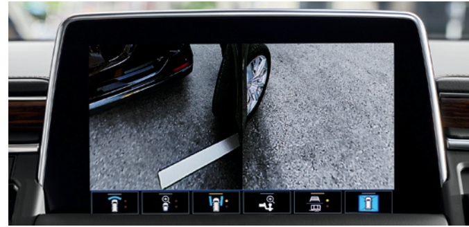
Front Side View Shows the position of the front tires when parking and during tight maneuvers.
