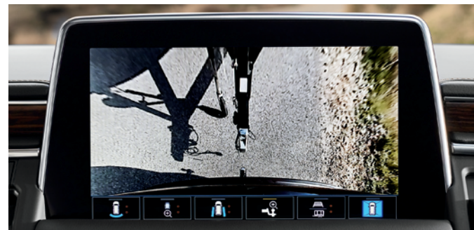
Hitch View Provides a close-up view of the receiver hitch to help with alignment when connecting to a trailer.
