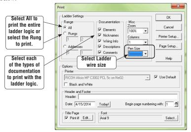
In this dialog, you can set the range to print all or any part of the ladder logic by either selecting **All**, **Rungs** or **Addresses** to be printed. Select any or all of the ladder documentation to print with the ladder logic. The **Miscellaneous** settings allows the level of zoom to print and the selection of the number of columns to print, also, the **Pen Size** allows the selection of the thickness of the pen used to draw wires, contacts, coils and boxes on high resolution printers.
