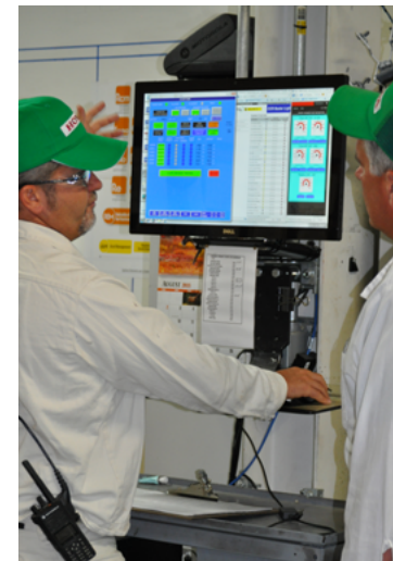
Honda Manufacturing of Indiana monitors its energy use in real time to identify equipment that can be turned off during breaks or between production shifts to meet energy-use targets.
