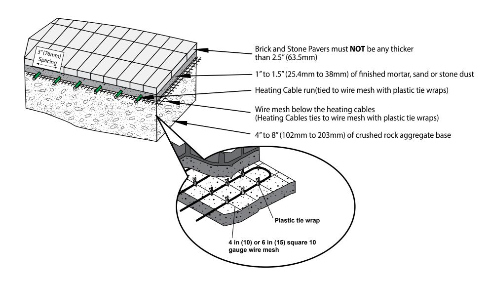
Note: Cables may be tied to reinforcement type mesh and then the mesh should be staked down to the base/crushed rock aggregate.
