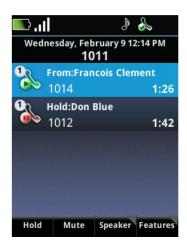
An active call has a light blue field when it is highlighted. An active call has a green field when another session cell is highlighted. Softkey presses affect highlighted cells. In the above example, you can see how the softkeys change when you highlight an active call.
