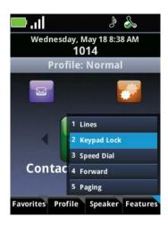
2 Press the 2 key or scroll to 2 Keypad Lock, and press the Yes softkey. Once you lock the keypad, all the keys become frozen except for an Unlock softkey, which replaces the Features softkey.
