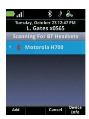
4 Locate your headset in the list and press the **Add** softkey to begin the acquire procedure. Once the handset has acquired the headset, the **Manage BT Headsets** screen appears with the headset displayed. The white icon indicates that it is paired but not connected.
