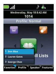
2 Scroll to a contact and press **Start** or press the contact index number, for example '1' on the keypad.
