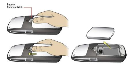
To replace the battery Pack, slide the tab of the Battery Pack into the bottom slot as shown below. Gently push the top of the Battery Pack until it snaps into place. You should not have to force it against the handset.
