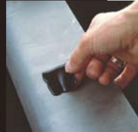
An operator dispenses RepliSet onto a sample, and then peels off the cured replica.
