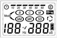
The LCD displays timer (10, 20, 30, 40, 50, 60 minutes and © continuous), function modes (B, C, M, MM, MR, SD), alternate mode, pulse rate, pulse width, battery low, and patient compliance meter.
