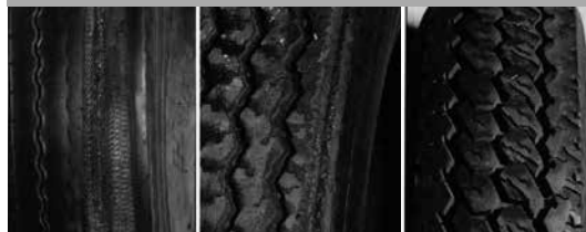
Flat spotting due to locked brakes
