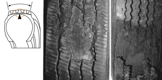
Bead damage due to curbing
