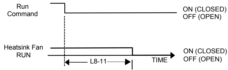
Fig. 84 Heatsink Cooling Fan Operation Timing Diagram
