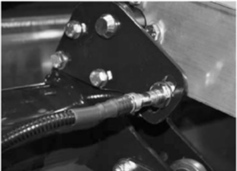
Sensor (E4) for sweeper position, backward
