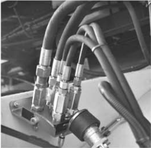
Multi-coupling on the combine harvester
