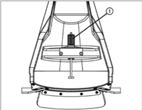
Set a distance of 2 cm from the ground by means of the screw
