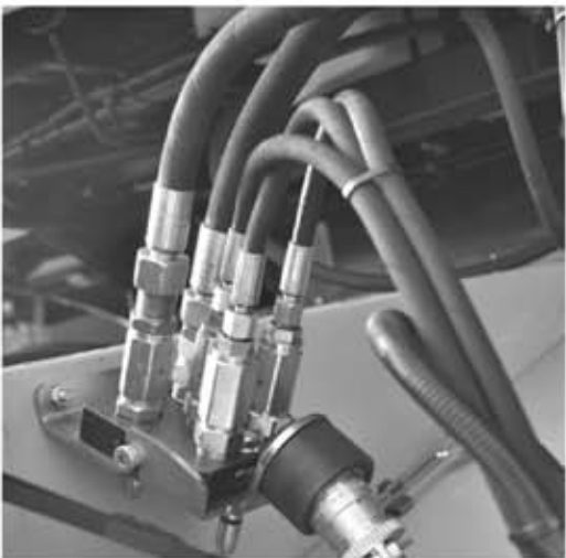
Multi-coupling on the combine harvester
