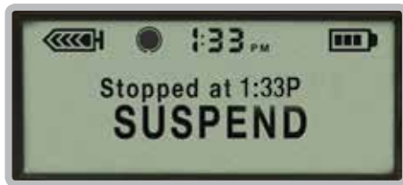
Pump in SUSPEND; notice the alarm icon
