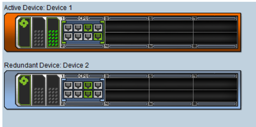
Figure 10-1: Mediant 4000 SBC HA Status Pane
