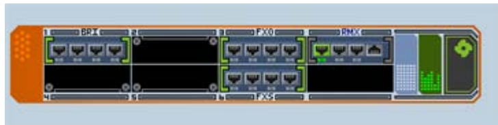
Figure 15-4: Mediant 1000B MSBR Status Pane
