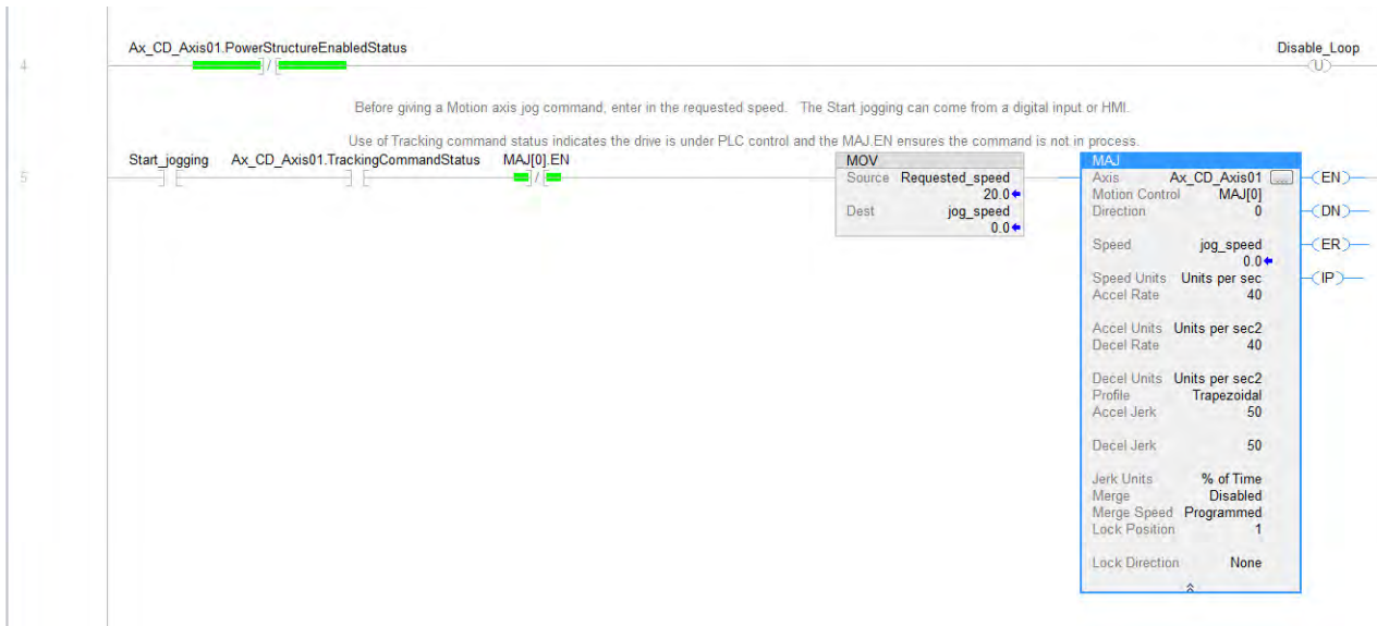
Figure 93 - Motion Instructions to Run the Motor at a Specific Velocity
