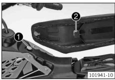
Hook the seat onto screw • and lower the seat at the rear while pushing it forward.
