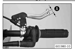
Push the handbrake lever forwards and check the play **A**.
