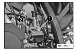
Screw in the idle adjusting screw ② until it stops and then to the prescribed basic setting.
