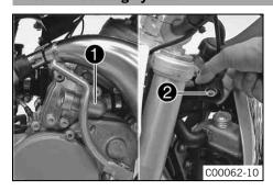
The water pump • in the engine forces the coolant to flow.
