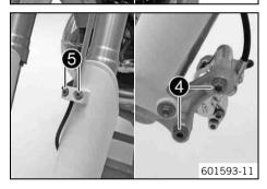
Position brake caliper, mount, and tighten screws 4.
