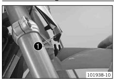
Position the fender with holding lugs • into the drill holes on the start number plate.
