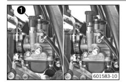
The choke knob **1** is fitted on the left of the carburetor.
