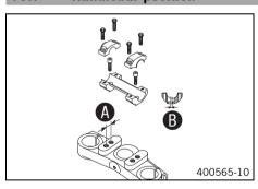
On the upper triple clamp, there are 2 holes at a distance of **1** to each other.
