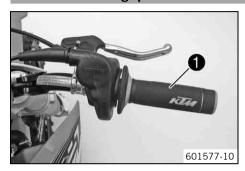
Throttle grip • is fitted on the right side of the handlebar.
