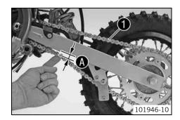
Push the chain at the end of the chain sliding component upward to measure the chain tension .
