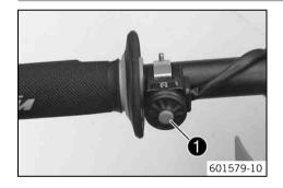
Kill switch **1** is fitted on the left side of the handlebar.
