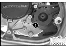
Remove gear oil level check screw ①.
