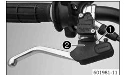
Position cover 2. Mount and tighten screw 1.
