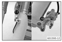
Position brake caliper, and mount and tighten screws **①**.
