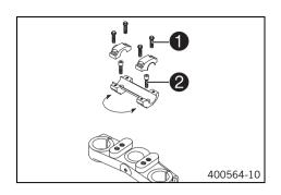
Remove the four screws ①. Remove the handlebar clamps. Remove the handlebar and lay it to one side.
