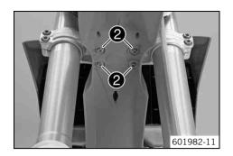
Position the front fender. Mount and tighten screws 2.
