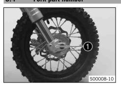
The fork part number **1** is stamped on the outside of the axle clamp.
