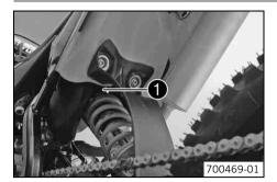
The shock absorber part number  $oldsymbol{0}$  is stamped on the top of the shock absorber above the adjusting ring towards the rear.
