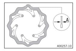
Check the thickness of the front and rear brake discs at several places on the disc to see if it conforms to measurement .
