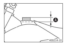
Fill the fuel tank with fuel up to measurement .
