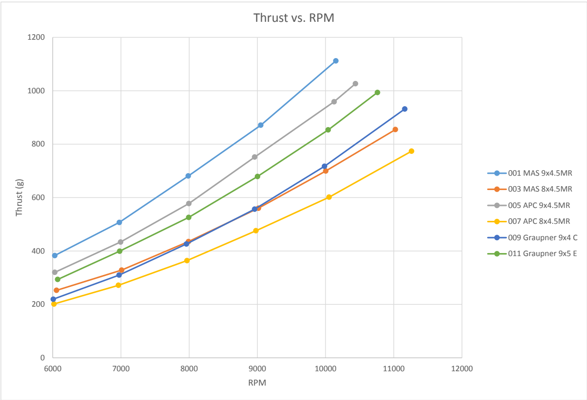
Figure 3 - Thrust vs. RPM with 900kv Motor
