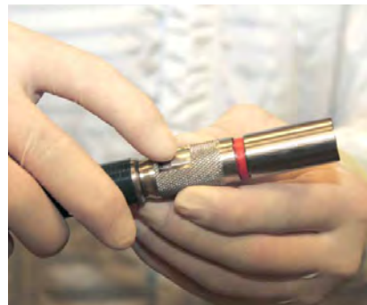
Figure 3.97. Sliding sleeve exposing red "not locked" indicator.
