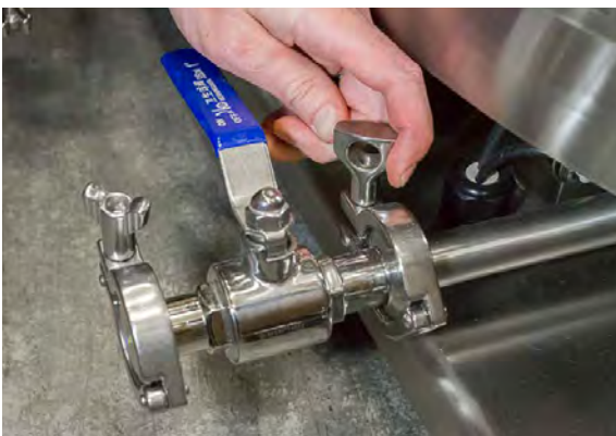
Figure 2.4. Attaching water jacket port using tri-clamp.
