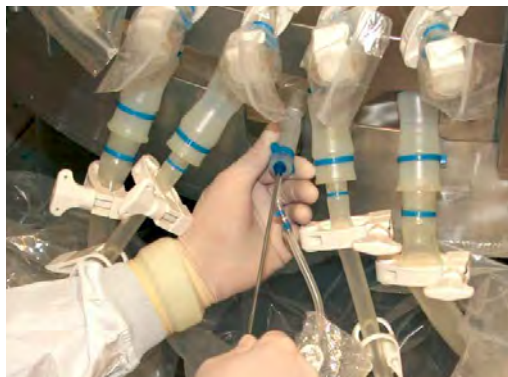
Figure 3.108. Insertion of the RTD into the thermowell.
