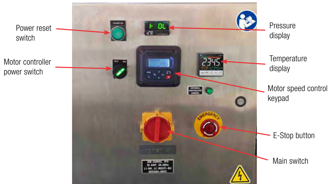
Figure 4.19. Front view of E-Box for 50–2,000 L S.U.B.s.
