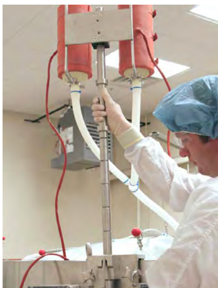
Figure 3.68. Raising the vent holder bracket.
