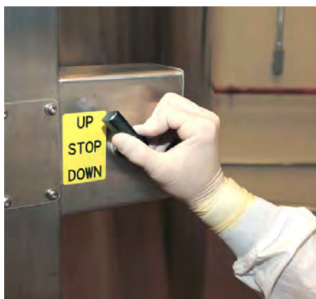
Figure 3.62. Operating the pneumatic lift control to raise the bag hoist.
