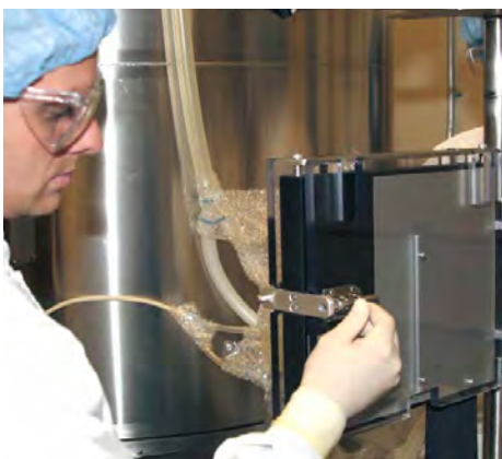
Figure 3.81. Opening the chiller plate doors.
