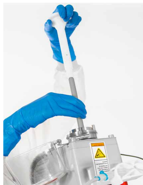
Figure 3.16. Twisting drive shaft to aid insertion.
