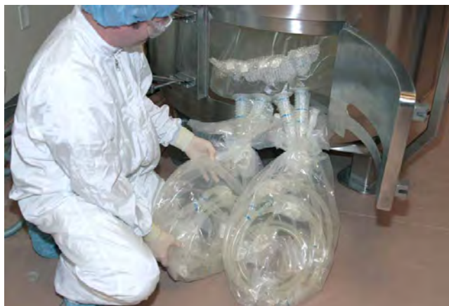
Figure 3.70. Feeding lines through the front access door.
