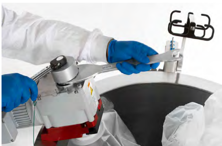
Figure 3.51. Tightening motor cap with wrenches.
