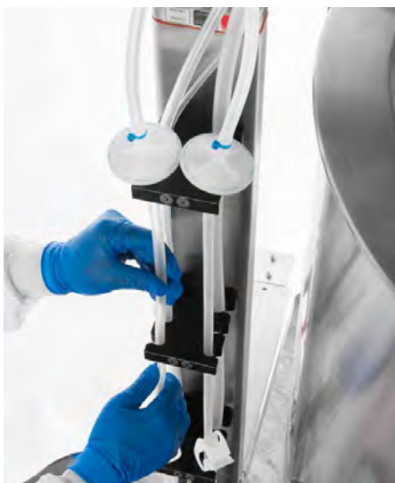
Figure 3.9. Inserting lines into the cable management system channels.
