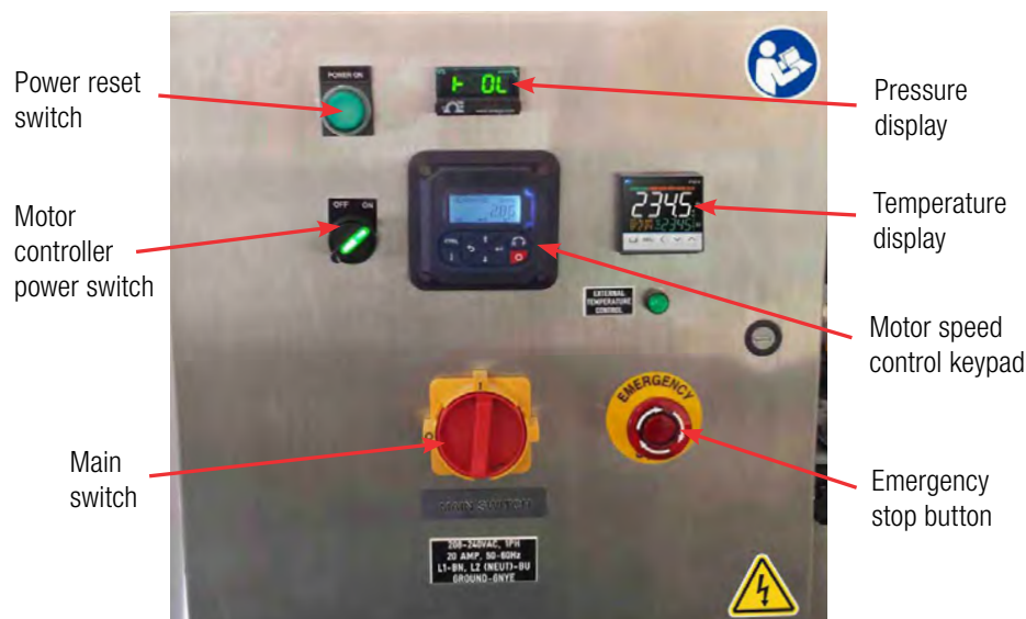
Figure 3.133. Front view of E-Box for 50–2,000 L S.U.B.s.
