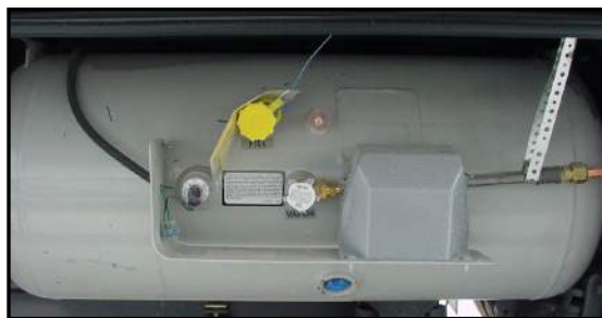
Figure 3-3. Liquid Propane Tank
