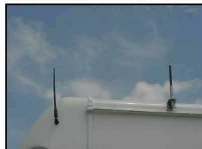
Figure 4-15. CB Antenna System
