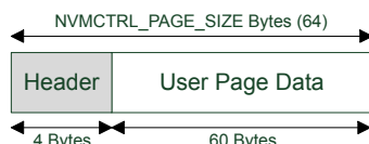
Figure 3-2 Internal Layout of An Emulated EEPROM Page
