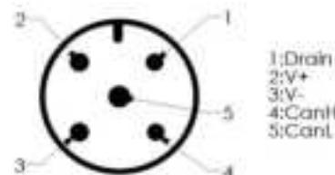
Figure 2-11 DeviceNet connector
