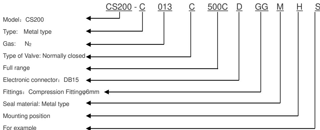
Customized requirement: In Chinese. Differential pressure, (0.3-0.5)MPa, customized fittings, customized calibration temperature, 40 °C
