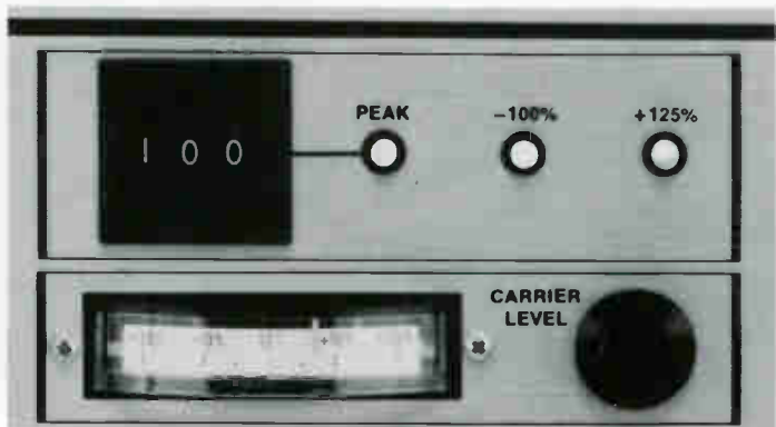
Digitally-settable Peak Flasher and Carrier Level Metering
