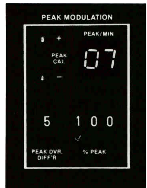
Figure 2: P.M.D.D. allows user to set peak width digitally.
