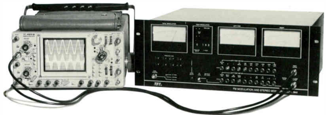
Figure 3: Model 844 permits front panel waveform monitoring.
