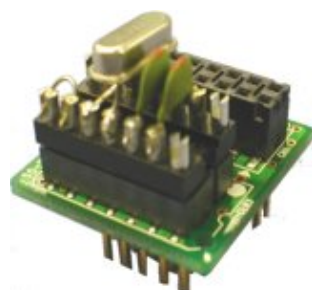
Figure 4-31. Appearance After Mounting Oscillator
