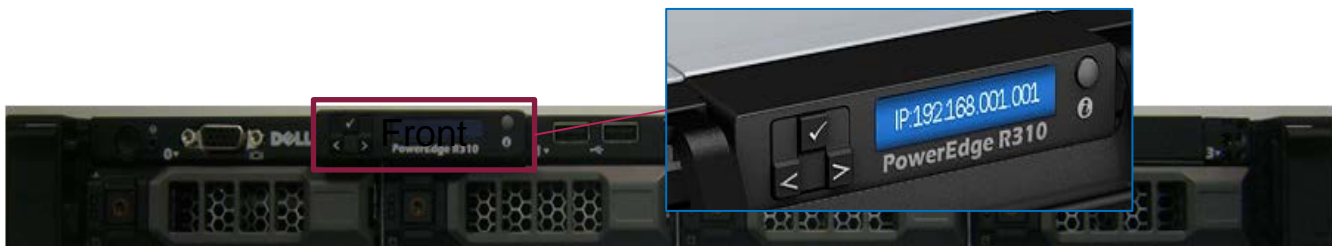
Figure 15. System Control Panel
