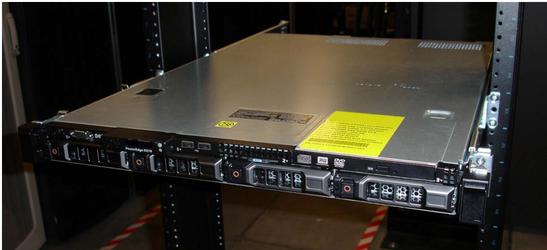
Figure 32. R310 Mounted in the A4 Static Rails in 2-post Center Mount Configuration
