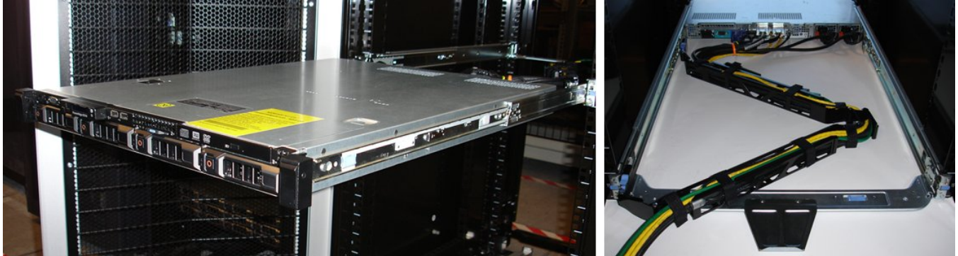
Figure 31. R310 Mounted in the A3 Sliding Rails with the CMA
