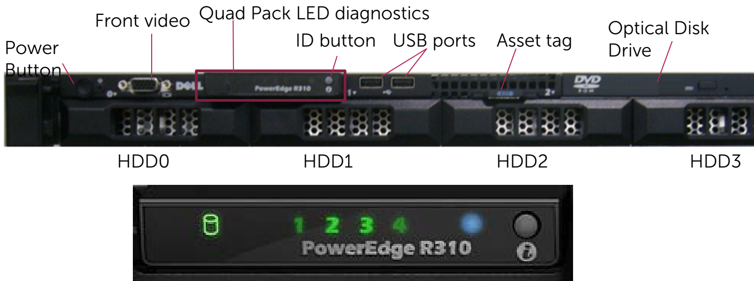
Figure 2. Front View Cabled HDD Configuration—With LED
