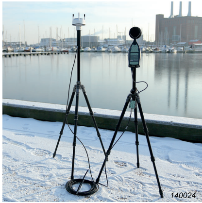
Fig. 8 Hand-held analyzer measuring outdoor noise using a weather station kit
