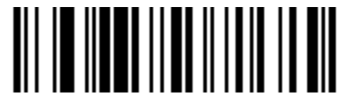
Message RTS/CTS Activate RTS before sending the first character and leave it active until after the last character has been transmitted.
