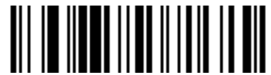
Message RTS/CTS Activate RTS before sending the first character and leave it active until after the last character has been transmitted.
