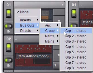
Assigning plug-in input source to a Group bus
