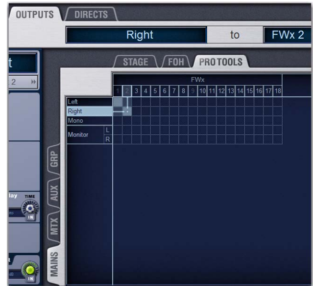
Routing the Mains bus to FWx channels for recording
