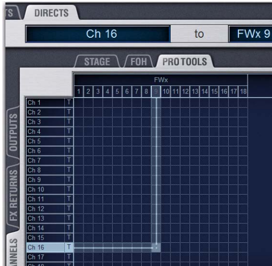
Routing a Direct Output to an FWx channel
