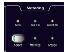
Bus output LEDs and Select switch
