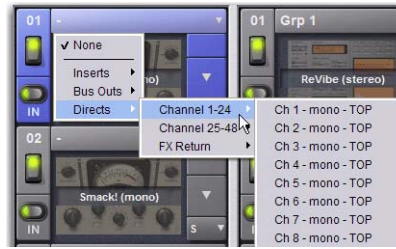
Assigning a channel Direct Out as a plug-in input source in the Plug-Ins page
