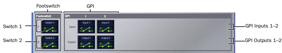
Figure 14. Footswitch and GPI Status Display in the Events window
