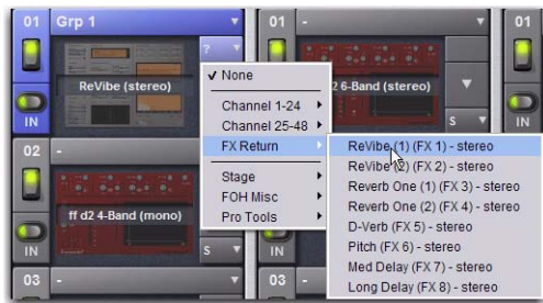
Assigning plug-in output to an FX Return
