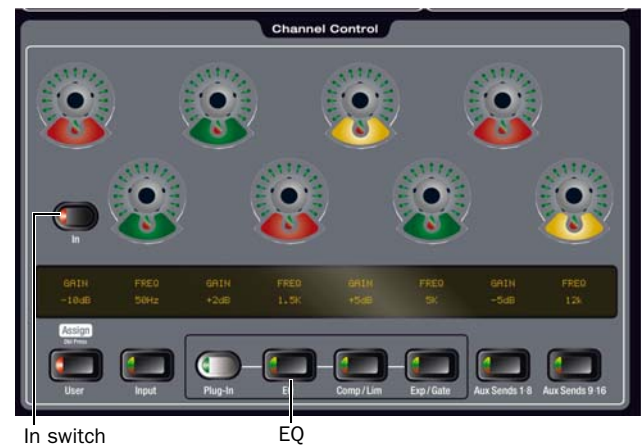
EQ switches in Channel Control
