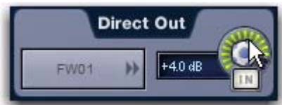
Adjusting Direct Output level from the Patchbay
