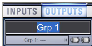
Changing the name of an Output channel in the Outputs page
