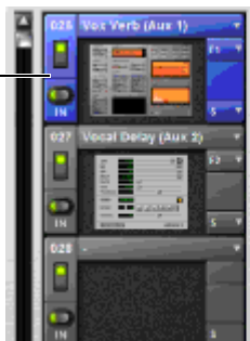
Highlighted rack slot indicating targeted plug-in
