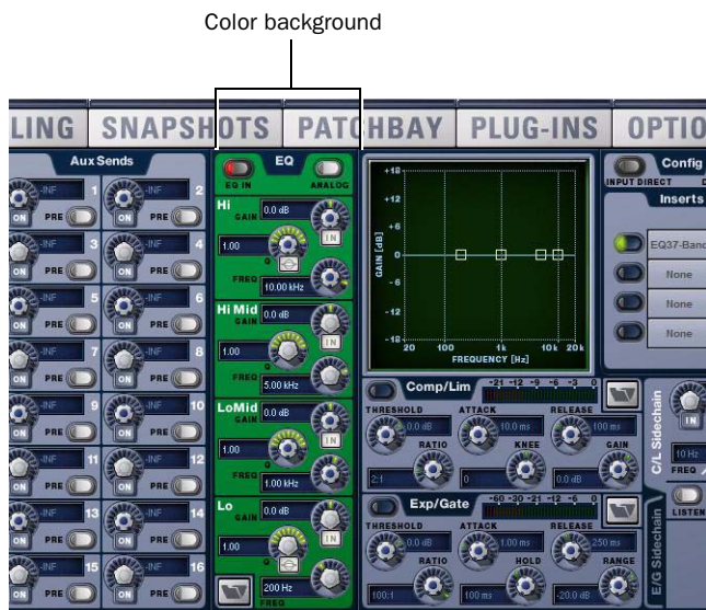
On-screen color indication of Channel Control function
