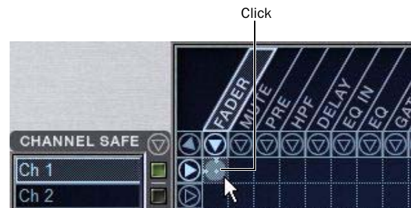
Enabling recall safe for channel 1 fader
