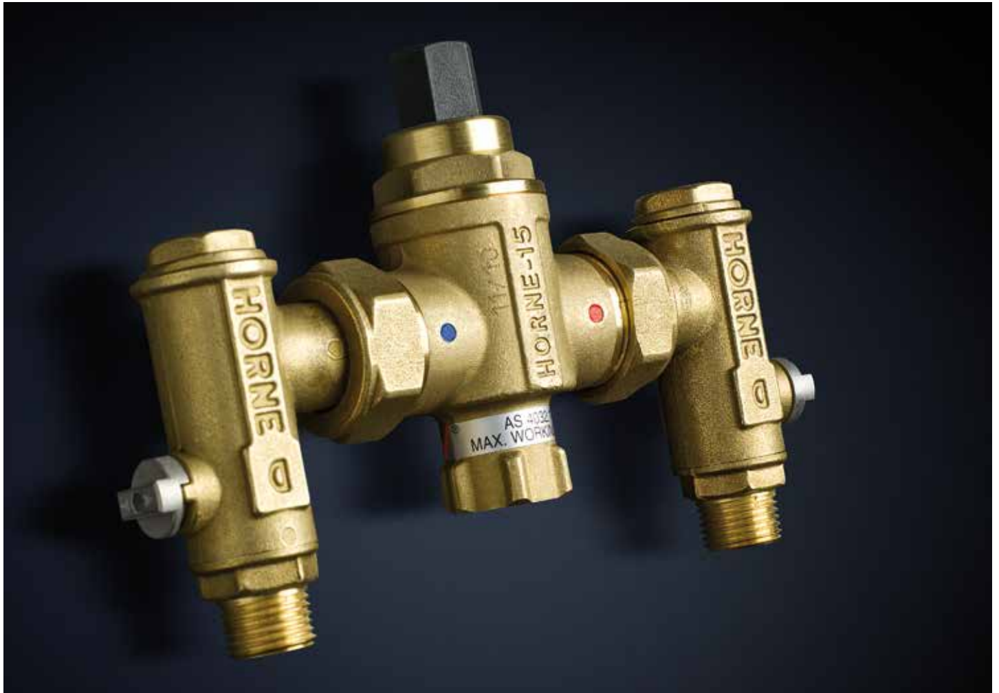
The HORNE TMV Model H1502. 42036 Thermostatic Mixing Valve. With 2 isolating valves, 2 strainers, 2 non-return valves.
