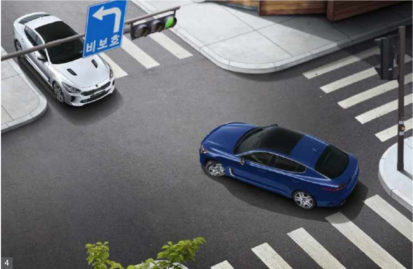
4 Forward Collision-avoidance Assist (FCA, oncoming traffic in intersections)
