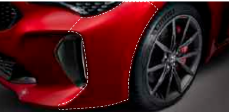
Vehicle protection film* Applied to the front and rear bumpers' sides, door edges, door caps, door steps, and fuel door.
