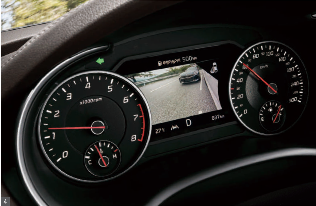
4 Blind-spot View Monitor (BVM) Cameras on the bottom of outside mirrors display a posterolateral view of the vehicle on the cluster's screen when the turn signal is activated, providing greater visibility of the surroundings in comparison to conventional outside mirrors for a safer driving environment.
