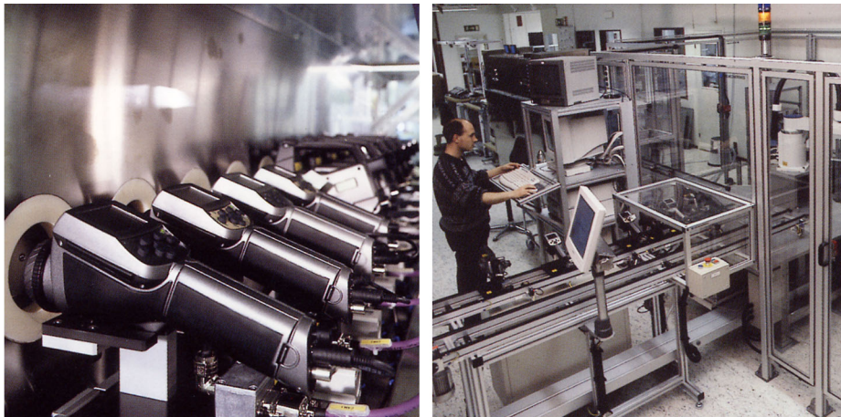
Figure 14.4 LEFT: Testing of IR cameras in the climatic chamber; RIGHT: Robot for camera testing and calibration.
