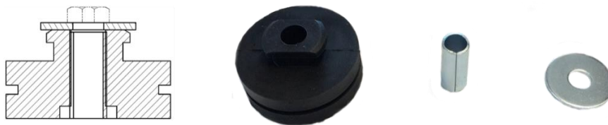
Figure 5: Mounting parts with sleeves and washers
