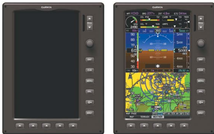
G300 Reversionary Mode (Failed PFD)
