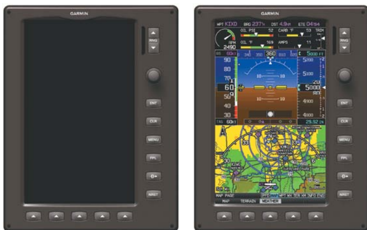
G300 Dual Display Reversionary Mode (Failed PFD)
