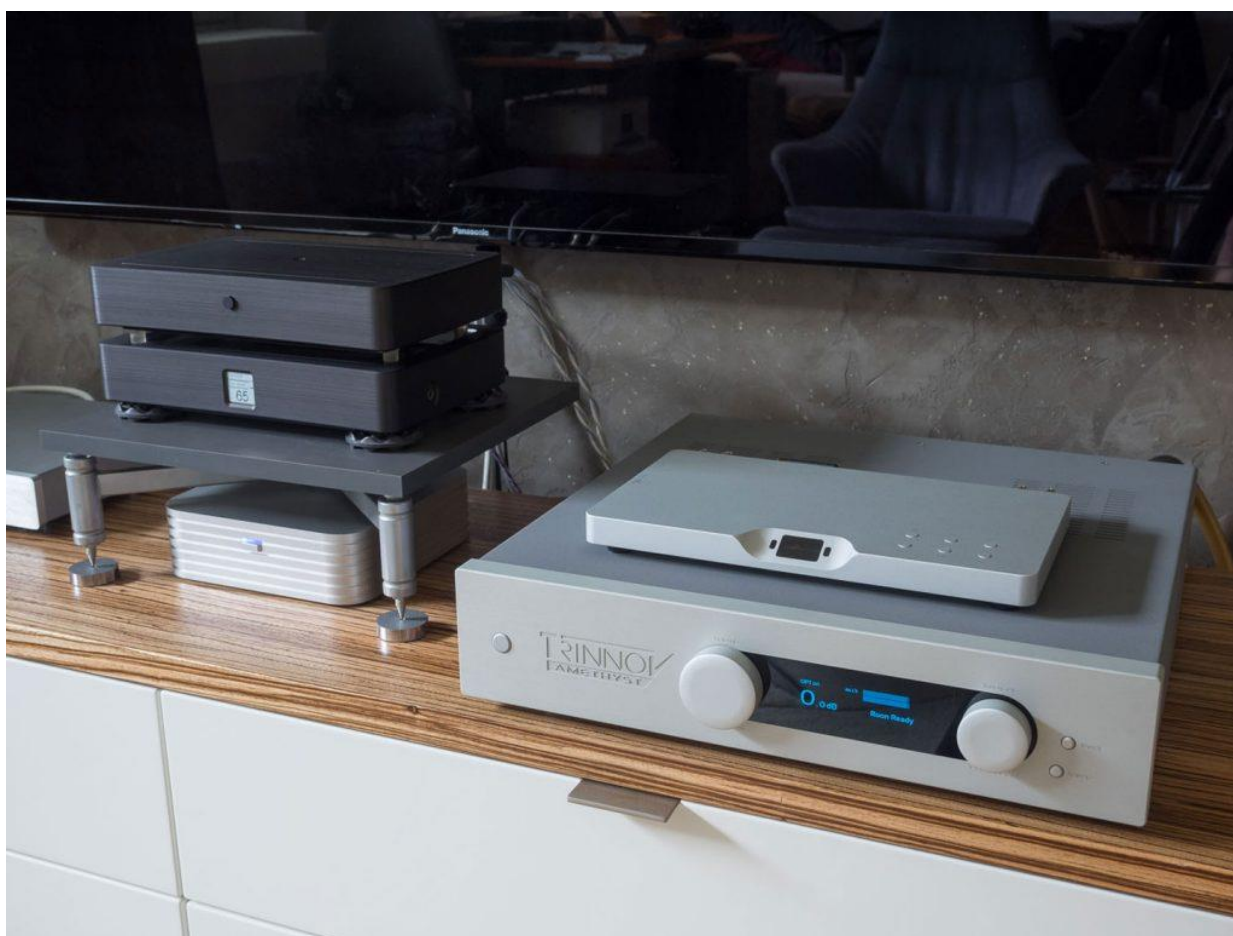
On the Trinnov Amethyst you see how small the Wslim is. Its footprint is similar to that of the Exogal components (black devices), but it is flat as a flounder and combines streaming, DAC, preamplifier and power amplifier in one housing (Photo: F. Borowski)
