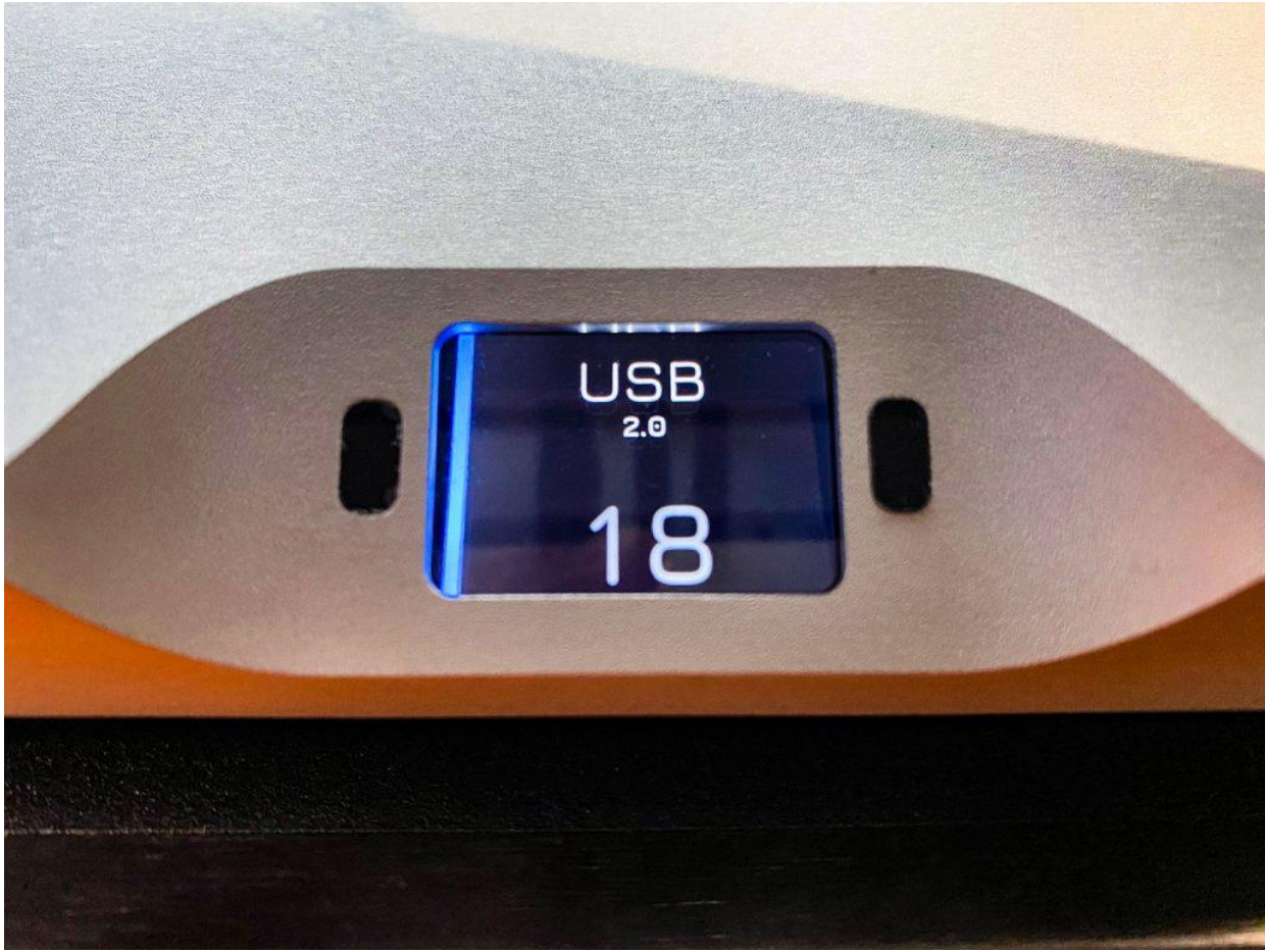
The small but high resolution and easy to read display. The strip on the left edge shows the playback status with colored codes. The "eyes" on the left and right are the IR receiver (Photo: F. Borowski)
