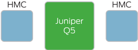
Figure 10: Juniper Q5 1 Tbps forwarding ASIC with 4 GB external memory using HMC technology
