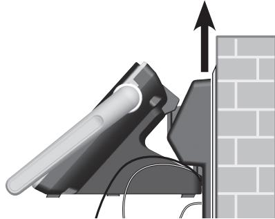
3. Unplug the telephone line cord or the DSL filter from the telephone wall jack. Push the telephone base up and away from the wall mount bracket to detach it from the wall mount bracket.
