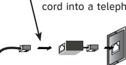
If you have DSL high-speed Internet service, a DSL filter (not included) is required. The DSL filter must be plugged into the telephone wall jack.
