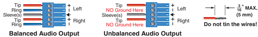
Figure 5. Audio Output Captive Screw Connector Wiring
