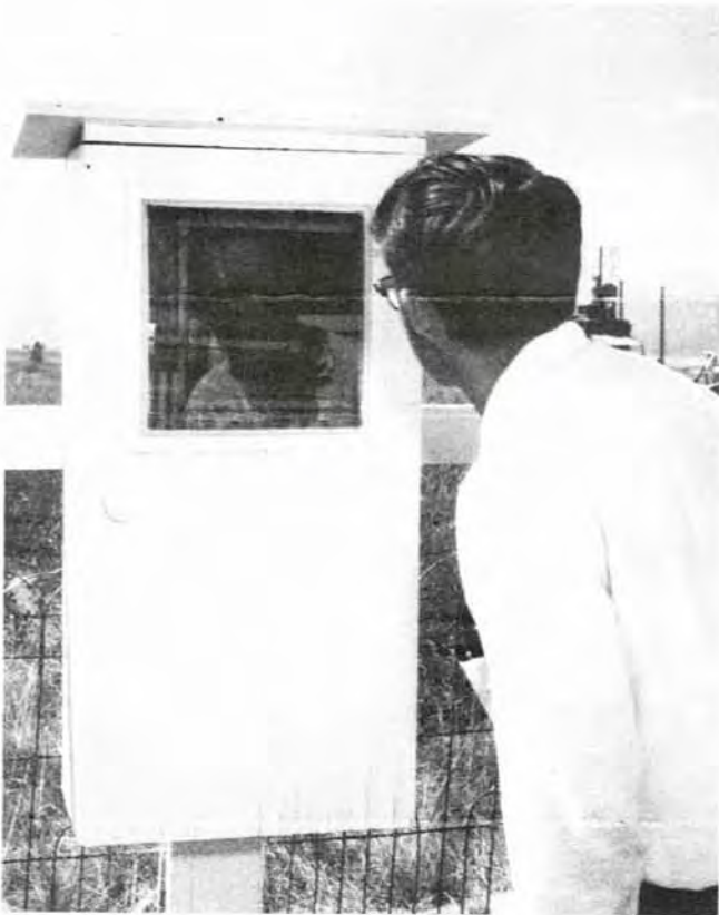
Figure 26.2 —Weighing the fuel moisture stick on Forester scale: top left, remove dust, dirt, etc.; top right, carefully hang stick on scale; bottom, close door to protect stick from wind.
