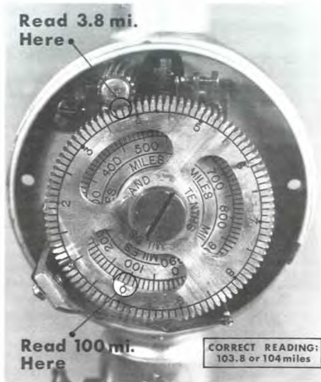
Figure 24.1—Detailed view of anemometer dial, indicating 104 miles of accumulated air movement past the anemometer cups.
