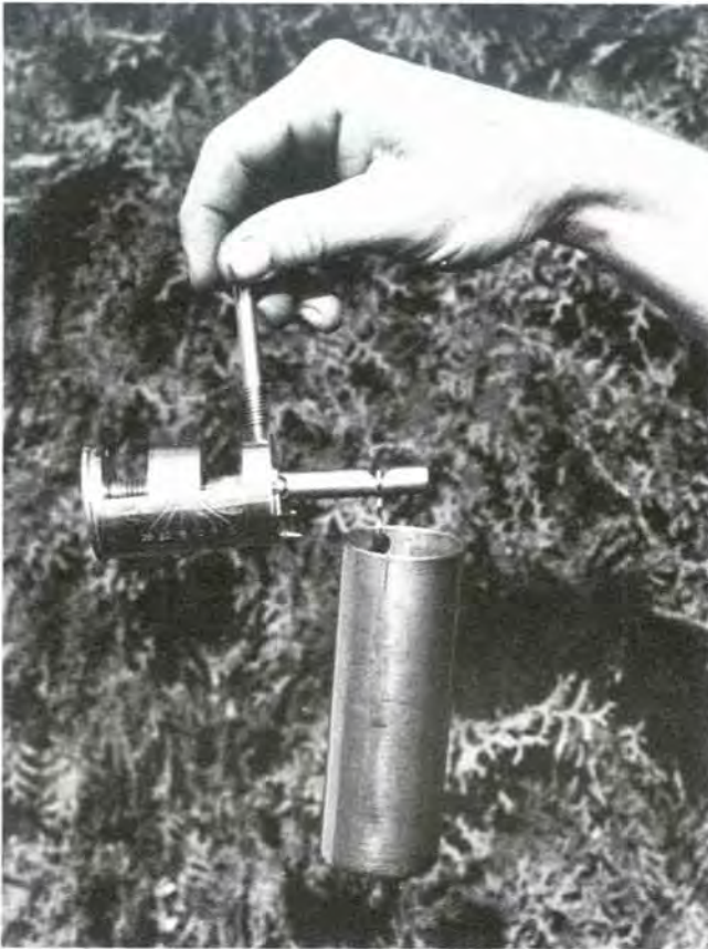
Figure 26.6—Checking calibration of Williams pocket scale, using cover as a 100-gram weight.
