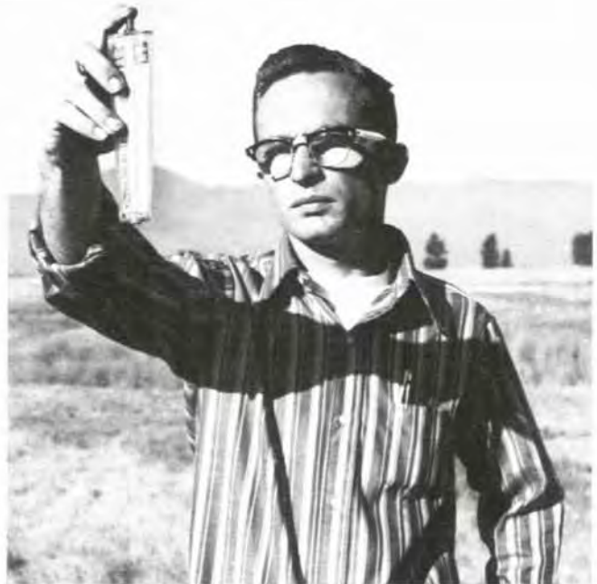
Figure 24.3 —To measure winds greater than 9 mi/h with Dwyer meter, face wind and cover top of stem with finger.
