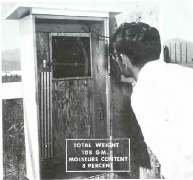
Figure 26.3 —Reading the Forester scale. The stick weighs 108 grams, compared with 100 grams oven-dry weight, so its moisture content is 8 percent as indicated by the pointer.
