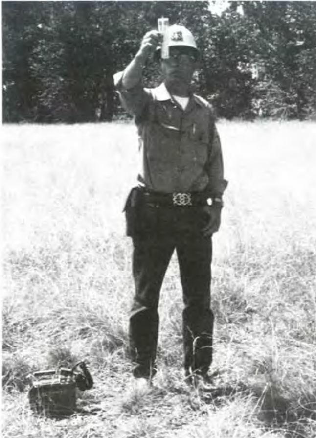
Figure 24.2 —Use of Dwyer hand-held wind meter, facing into wind. Keep fingers clear of top stem when measuring winds less than 10 mi/h.
