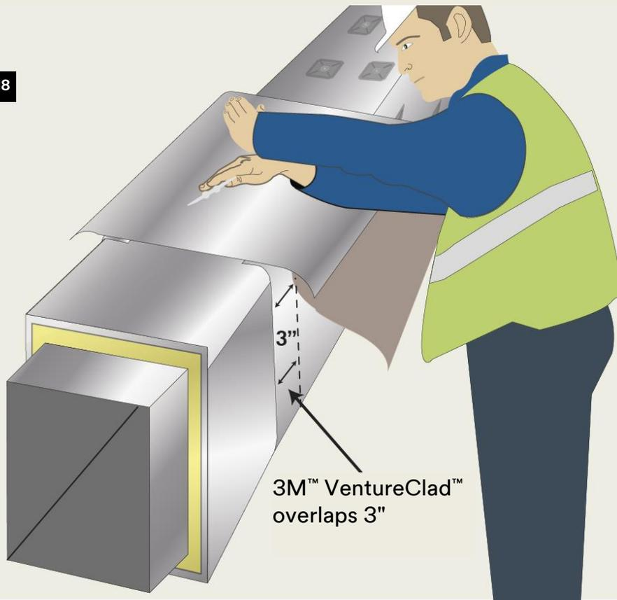
*Figure 18 shows the insulator applying 3M™ VentureClad™ to the next section of duct. Note that he will overlap the first section's 3M™ VentureClad™ by 3 inches (75mm). Note that the installer should have first covered the speed washers with pieces of 3 inch x 3 inch (75mm x 75mm) 3M™ Venture Tape™, as shown in Figure 2.*
