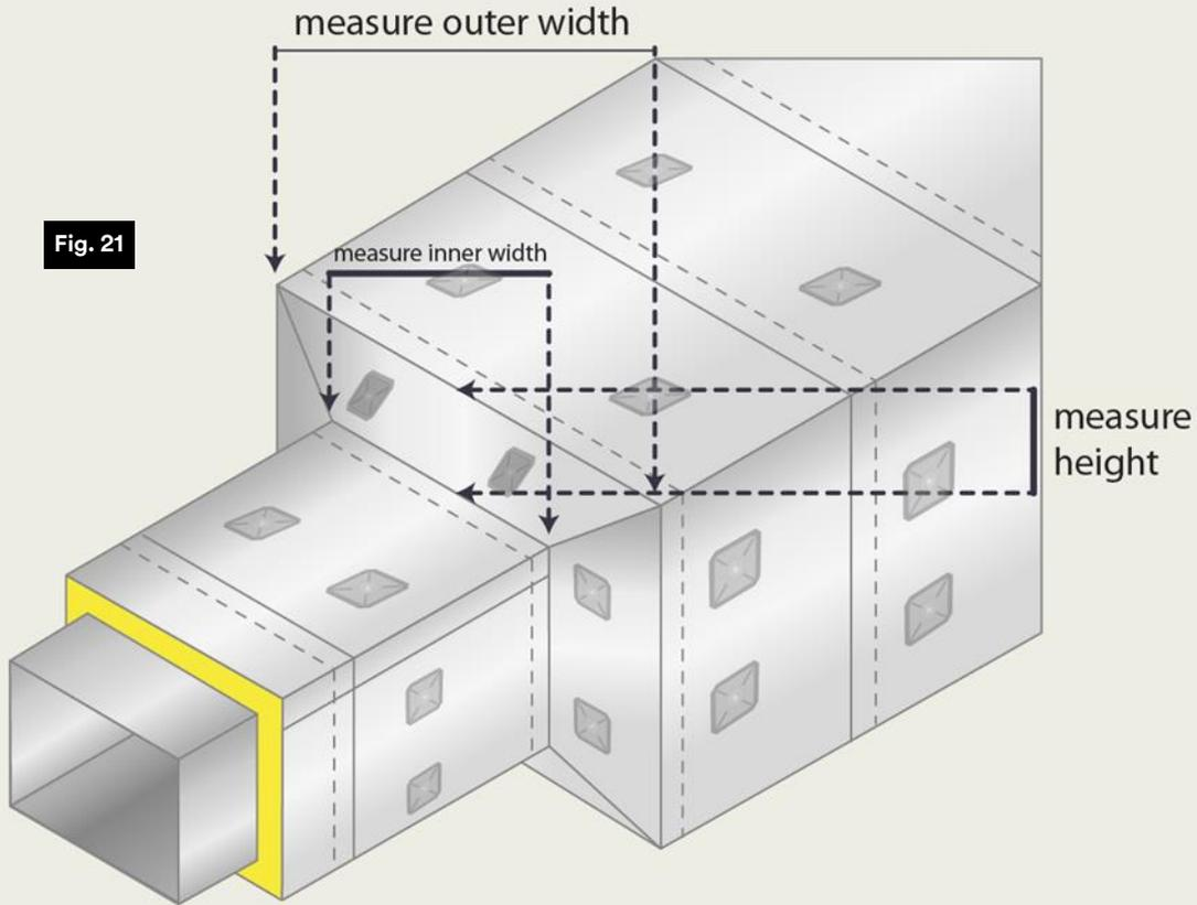
Figure 21 shows where to make measurements for the 3M™ VentureClad™ sections that will be applied to the insulated duct reducer sections.
