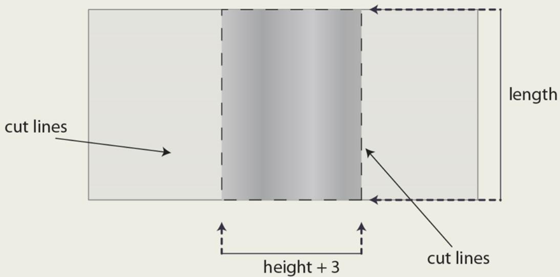
*Figure 32 shows cut lines for cutting a piece of 3M™ VentureClad™ for each of the two sides of the smaller insulated rectangular ducts that connects to the insulated reducer. The extra 3 inches (75mm) added to the height allows for the 3M™ VentureClad™ application to start on the top surface before being applied to the sides.*
