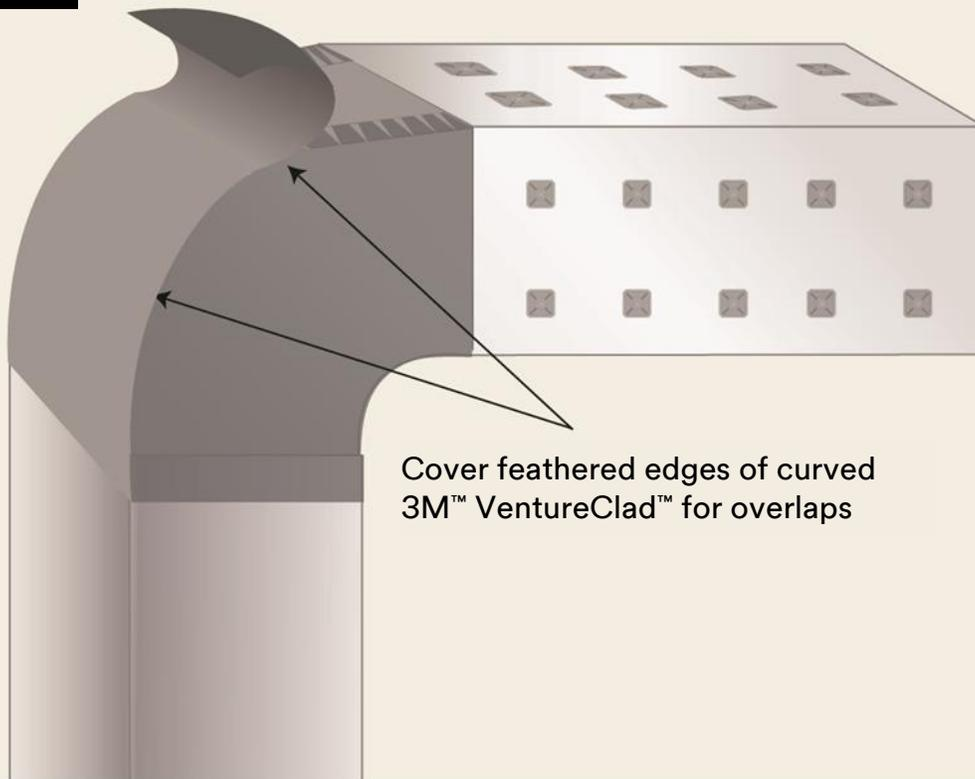
Figure 51 shows the top side of the insulated rectangular duct covered with the cut piece of 3M™ VentureClad™ Section 4.
