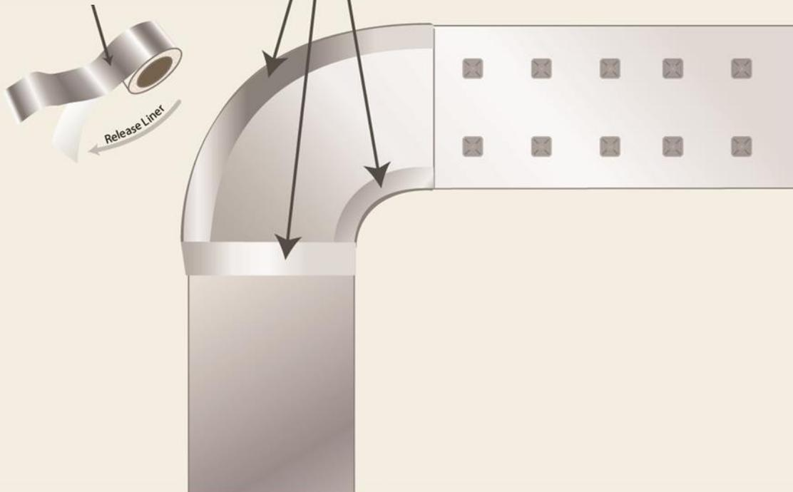
*Figure 52 shows the insulated, 90° rectangular duct elbow totally covered with 3M™ VentureClad™. Note that the heel and throat edges, as well as the butt joint between the straight rectangular duct and the elbow, must all be sealed with 3M™ Venture Tape™ (either 1577CW or 1578CW). Feather the 3M™ Venture Tape™ as necessary to get it to lay down on the elbow sides.*
