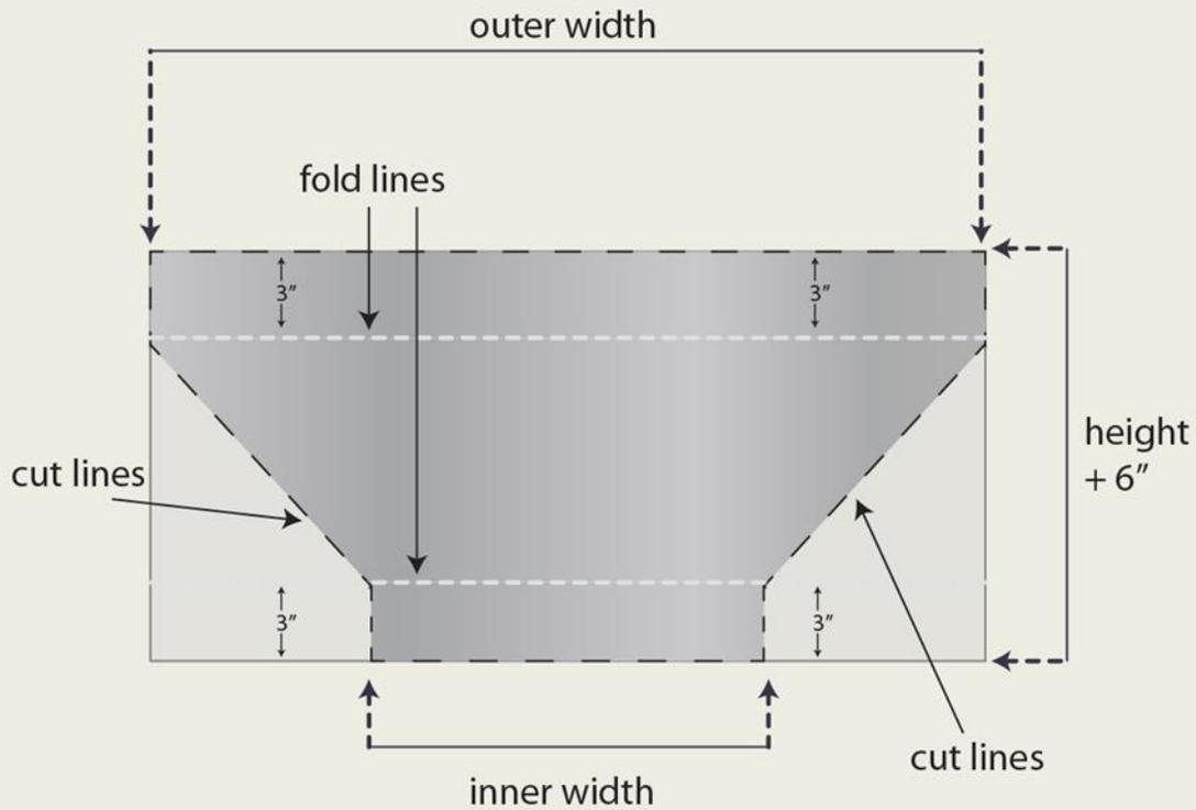
Figure 22 shows where to make cuts to the 3M™ VentureClad™ used to cover the bottom and top faces of the insulated duct reducer. Note that the installer should first start with a rectangular section measuring outer width x height + 6 inches (150mm), then mark the cut lines, and finally cut along the cut lines.
