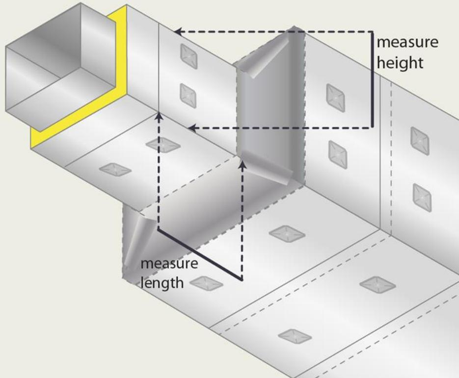
Figure 31 shows measurements to be made on the sides of the smaller insulated rectangular ducts.
