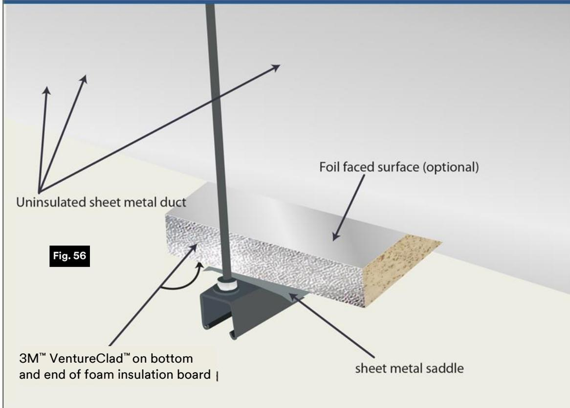
*Figure 56: 3M recommends that at least two installers slide the faced insulation board between the sheet metal duct and the duct hanger + sheet metal saddle, with the 3M™ VentureClad™ facing down towards the saddle. Be certain to center this faced insulation board. Notice that the insulation board is wider than the sheet metal duct by 2 x insulation thickness (or by 1 x insulation thickness on each side).*
