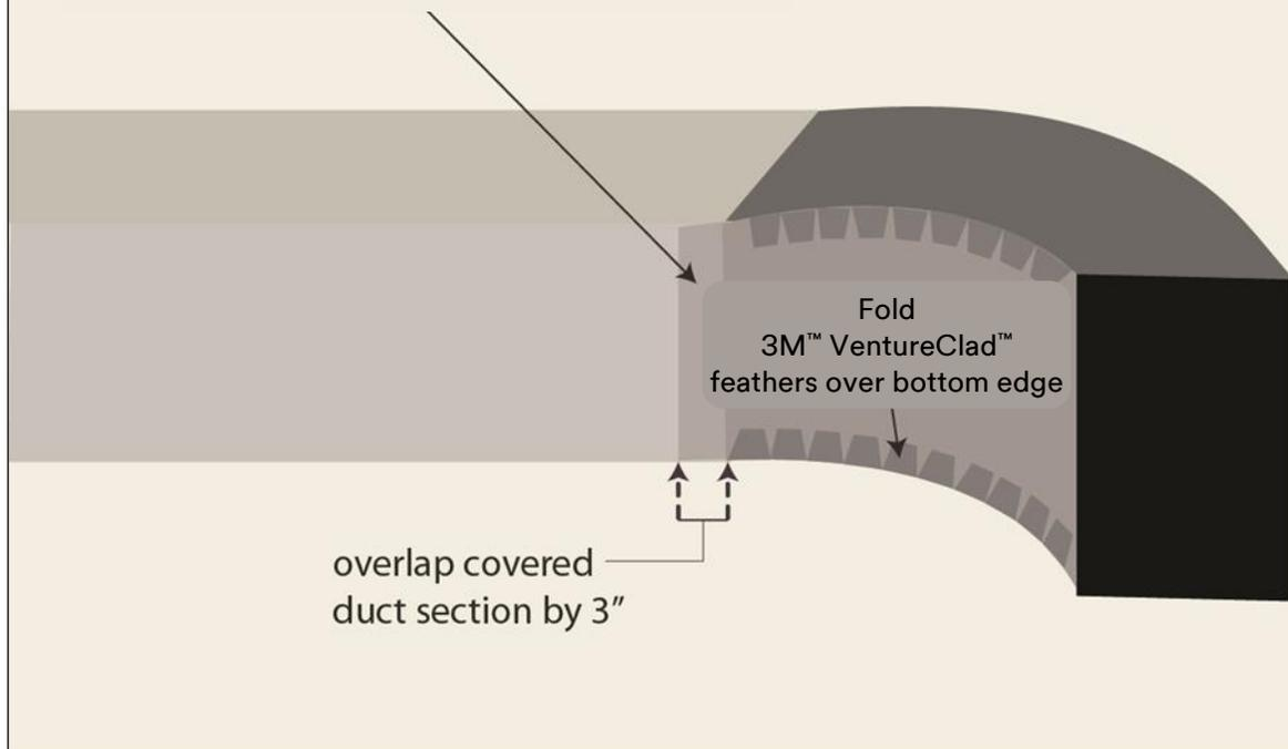
Figure 47 shows the elbow throat covered with a specially cut rectangular section of 3M™ VentureClad™ to the elbow heel: Section 3. This Section 3 will cover the “feathers” from Sections 1 and 2.
