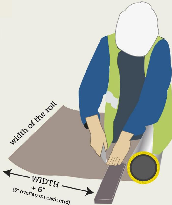
Figure 4 shows an installer cutting a sheet of 3M™ VentureClad™ from the roll. In this case, the sheet dimensions will be the width of the roll x the width of the insulated duct. This cut sheet will be applied to the bottom of the insulated duct after first removing several inches of the release liner. Note the 3 inch (75mm) overlaps and hence the 6 inches (150mm) greater length).
