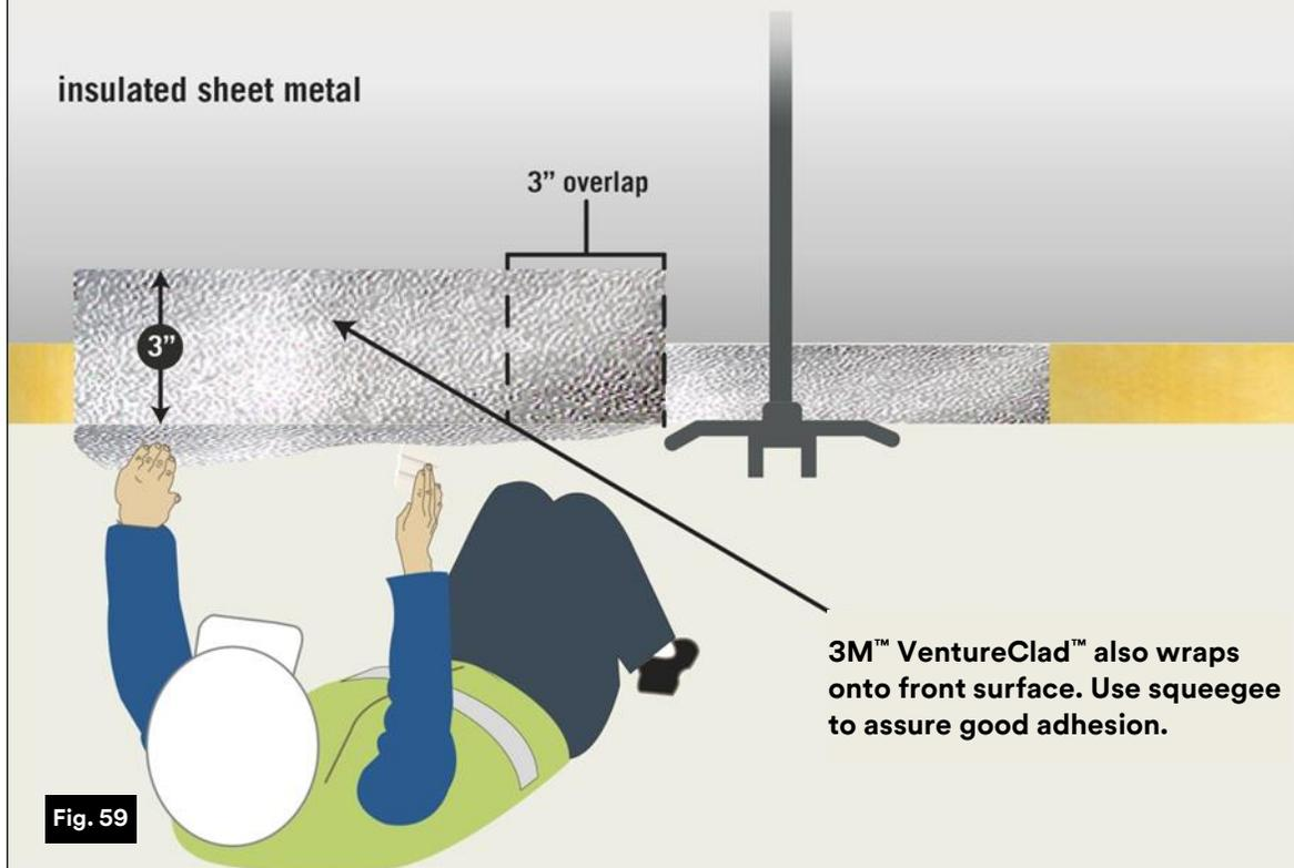
*Figure 59: 3M recommends the installer use a squeegee to get a complete adhesion of the 3M™ VentureClad™ to the bottom surfaces of the insulation board. Also use the squeegee to assure good adhesion to the duct sides, as show in the drawing above.*
