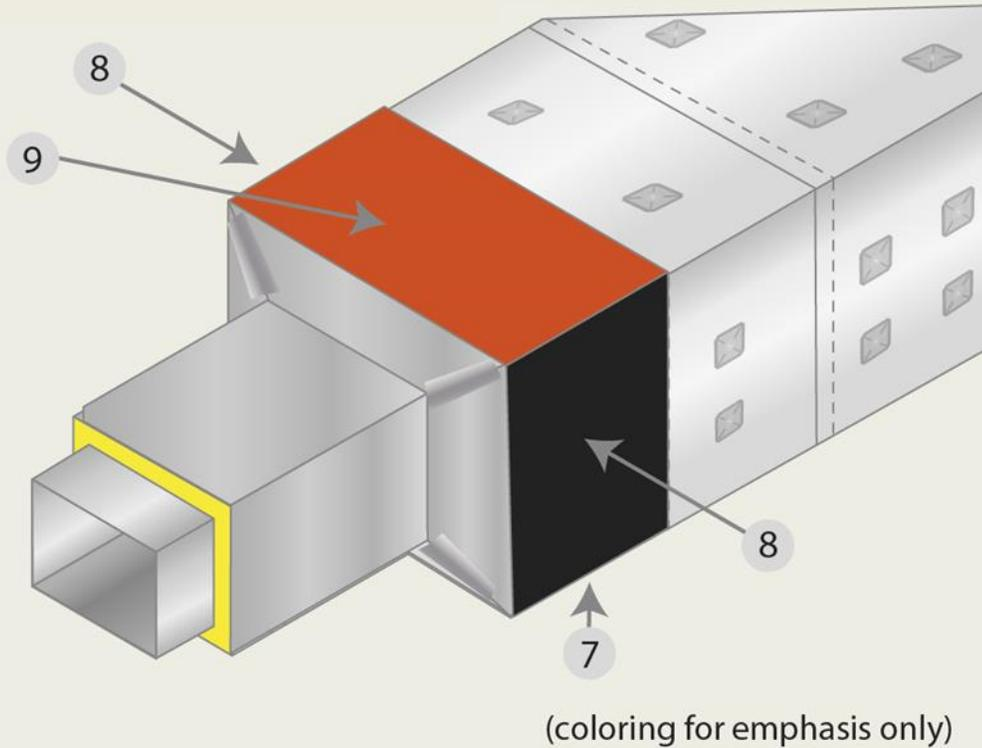
*Figure 38 shows the first two pieces of 3M™ VentureClad™ to be applied to the surfaces of the larger insulated rectangular duct that connects to the reducer. First, apply the 3M™ VentureClad™ to the bottom (# 7), then apply it to each of the two sides (# 8), and finally apply it to the top (# 9).*
