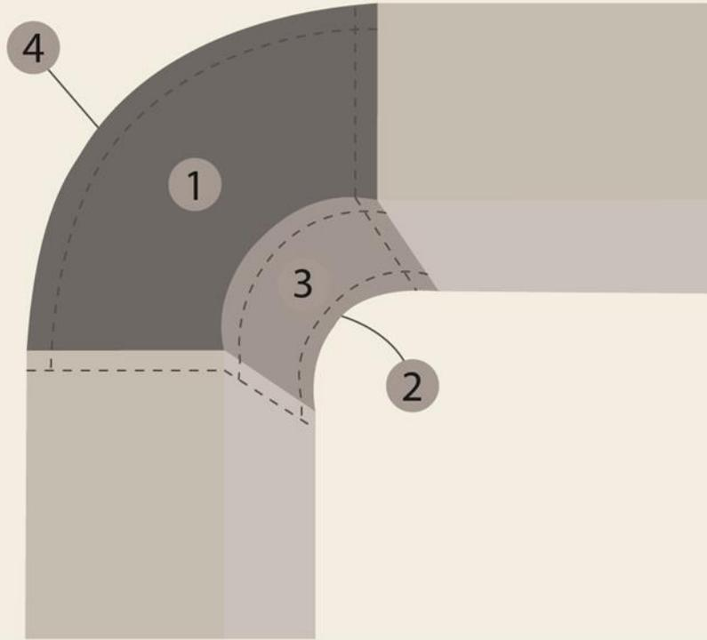
Figure 42 shows the sequence for covering the 90° insulated rectangular elbow with 3M™ VentureClad™ for a horizontal duct with 4 pieces of cut 3M™ VentureClad™. Hence, each rectangular elbow has two sides (Sections 1 and 2), a bottom or throat (Section 3) and a top or heel (Section 4). In the case of one vertical duct transitioning to a horizontal duct, the sequence is the same.
