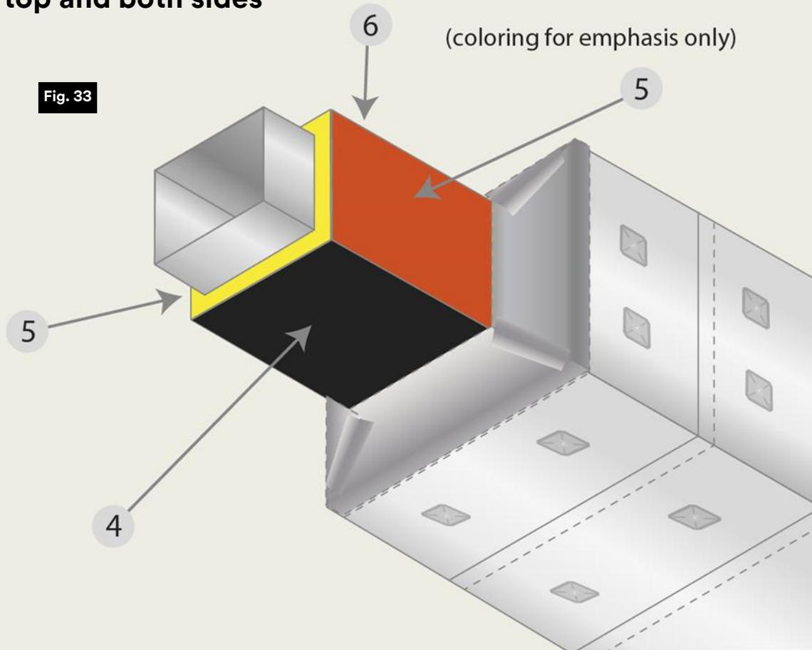
*Figure 33 shows the application of the two cut 3M™ VentureClad™ pieces, first to the bottom of the smaller rectangular duct (# 4), then to one of the two vertical sides (# 5), and finally the top (# 6).*
