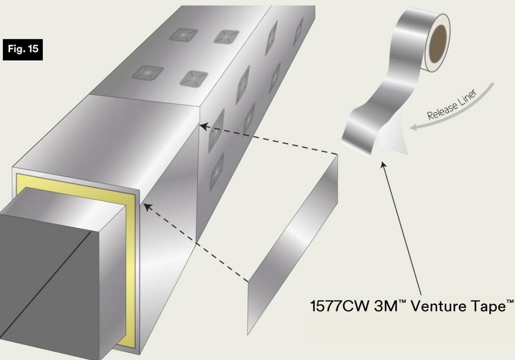
*Figure 15 shows the location where a cut strip of 4 inch (100mm) wide 1577CW 3M™ Venture Tape™ will be applied to reinforce one of the 3M™ VentureClad™ 1579GCW joints. This step is unnecessary when using the lighter weight 1577CW 3M™ VentureClad™. Note that the more flexible 1578CW 3M™ Venture Tape™ may also be used to seal the 3M™ VentureClad™ seams.*
