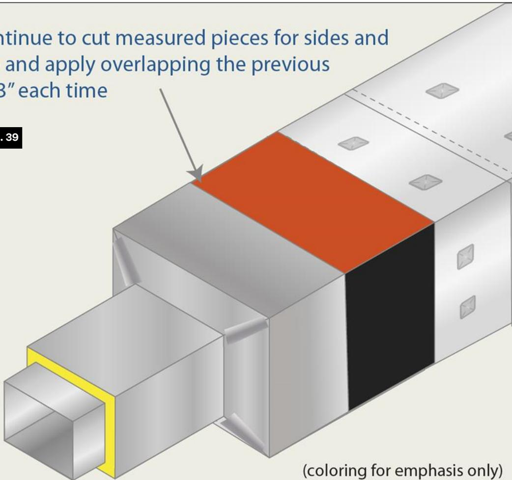
Figure 39 shows where the next pieces of 3M™ VentureClad™ are to be applied on the larger section of the insulated rectangular duct that connects to the reducer.
