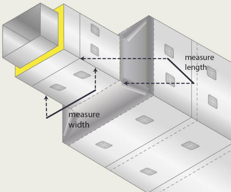
Figure 29 shows measurements to be made of the smaller of the two insulated rectangular ducts that connects to the reducer.
