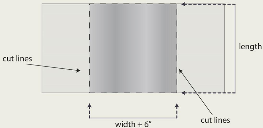
Figure 30 shows the cuts to be made to the 3M™ VentureClad™ to cover the bottom of the smaller insulated rectangular duct. In this case, “length” may be the 3M™ VentureClad™ roll width. The extra 6 inches (150mm) on the width allows the 3M™ VentureClad™ to be folded, by 3 inches (75mm), over each of the two vertical sides.
