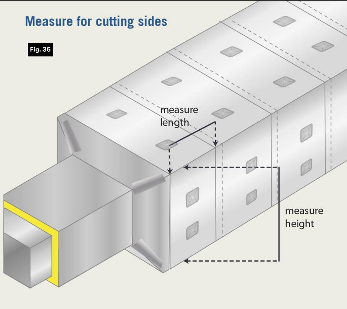
Figure 36 shows measurements to be made on the sides of the larger insulated rectangular duct that connects to the reducer.
