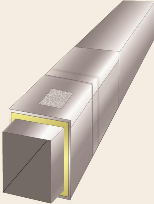
*Figure 63: Press the piece of 3M™ Venture Tape™ over the rip or tear, being certain to cover the damaged portion of the 3M™ VentureClad™. Run a squeegee over the repair to make certain that the 3M™ Venture Tape™ is firmly adhered to the 3M™ VentureClad™. Note that either 1577CW 3M™ Venture Tape™ or the more flexible 1578CW 3M™ Venture Tape™ may also be used to make these repairs.*
