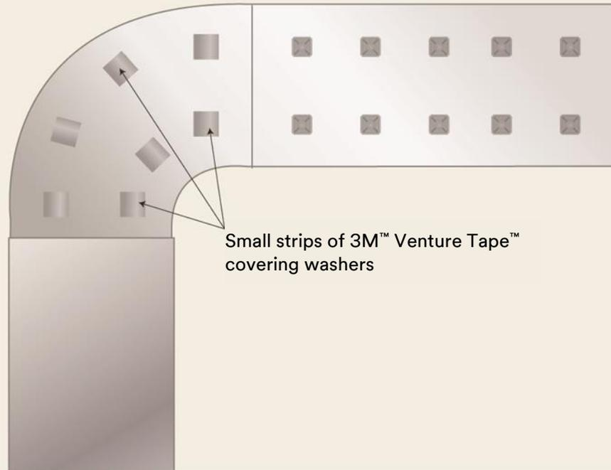
*Figure 43 shows small strips of 3M™ Venture Tape™, such as 1525CW FSK, used to first cover the exposed pins and washers that are holding the insulation board to the duct.*
