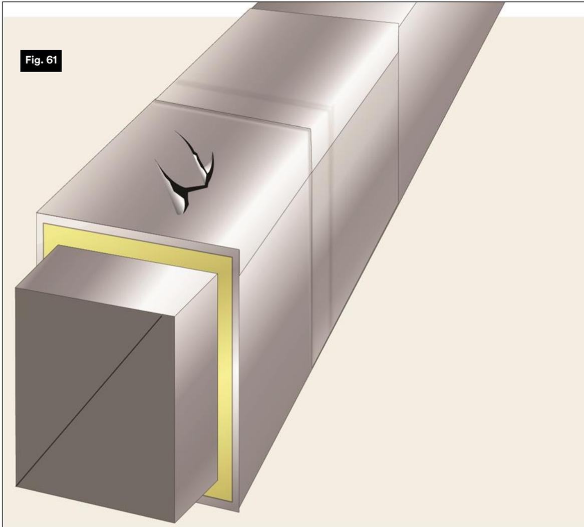
*Figure 61: Sometimes the 3M™ VentureClad™ on a duct develops a rip or tear. When it does so, it should be repaired as soon as possible using 3M™ Venture Tape™. Fortunately, doing so is relatively easy.*
