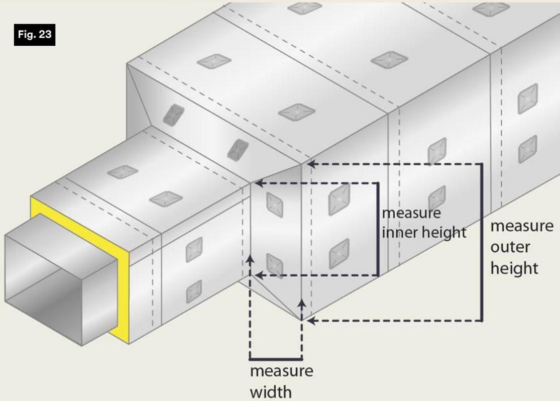
Figure 23 shows where to make measurements for the 3M™ VentureClad™ to be applied to the left and right sides.
