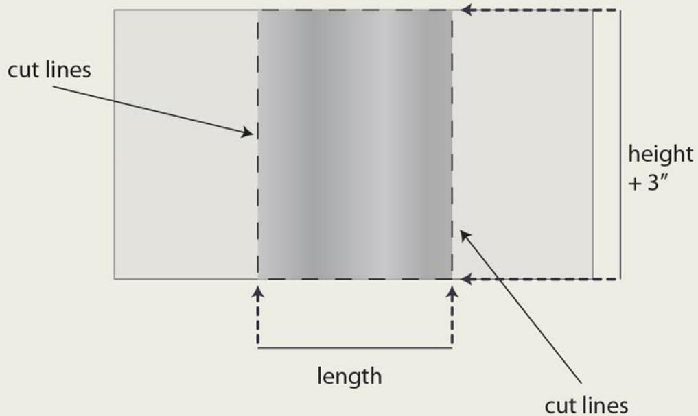
Figure 37 shows cut lines for cutting the two sidewall pieces of 3M™ VentureClad™ to cover the larger insulated rectangular duct. Note that the extra 3 inches (75mm), added to the height, allows for the 3M™ VentureClad™ to start on the top surface and then be folded over to cover the sidewall. Also, note that “length” may simply be equal to the width of the 3M™ VentureClad™ roll.
