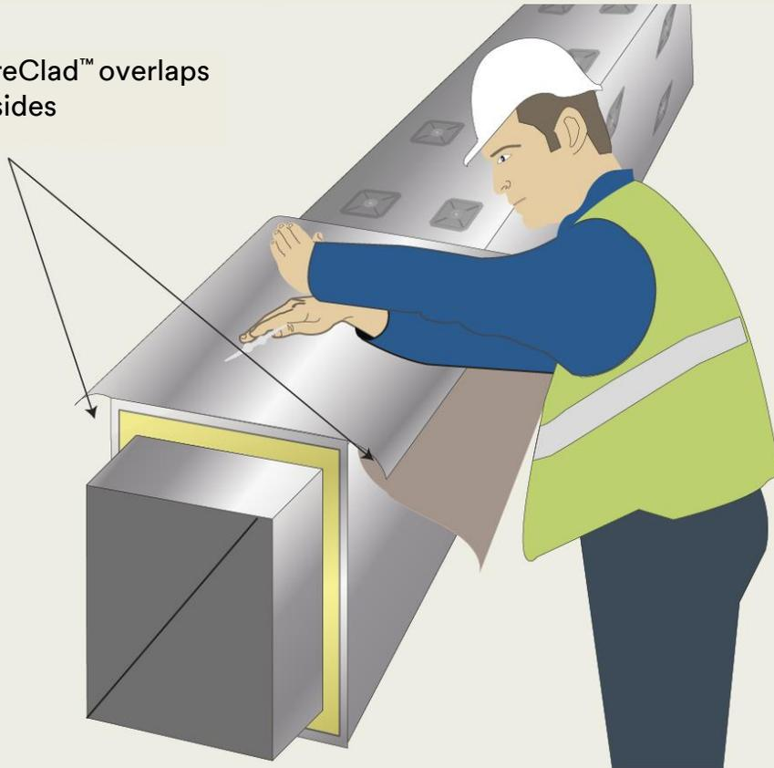
*Figure 14 shows the installer using the squeegee to smooth out the 3M™ VentureClad™ and to assure himself that the 3M™ VentureClad™ has completely adhered to the top surface of the insulated duct (piece 4).*
