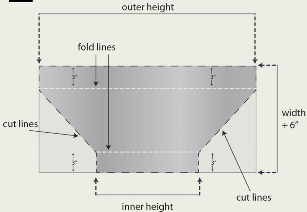
*Figure 24 is similar to Figure 18 except this is for the two side pieces of 3M™ VentureClad™ that are to be applied to the left and right sides of the insulated rectangular duct reducer.*
