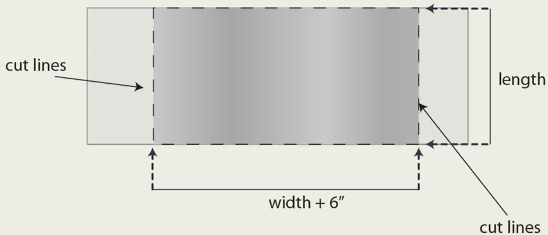
Figure 35 shows the cut lines for the bottom and top pieces of 3M™ VentureClad™ to be applied to the larger insulated rectangular duct section connecting to a reducer. The dimension on the drawing shown as “length” may simply be the 3M™ VentureClad™ roll width. The extra 6 inches (150mm), added to the dimension “width”, allows for a 3 inch (75mm) overlap of each of the two vertical sides.
