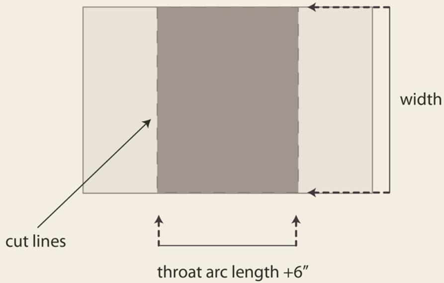
Figure 49 shows the rectangular piece of 3M™ VentureClad™ cut to fit the throat Section 3.
