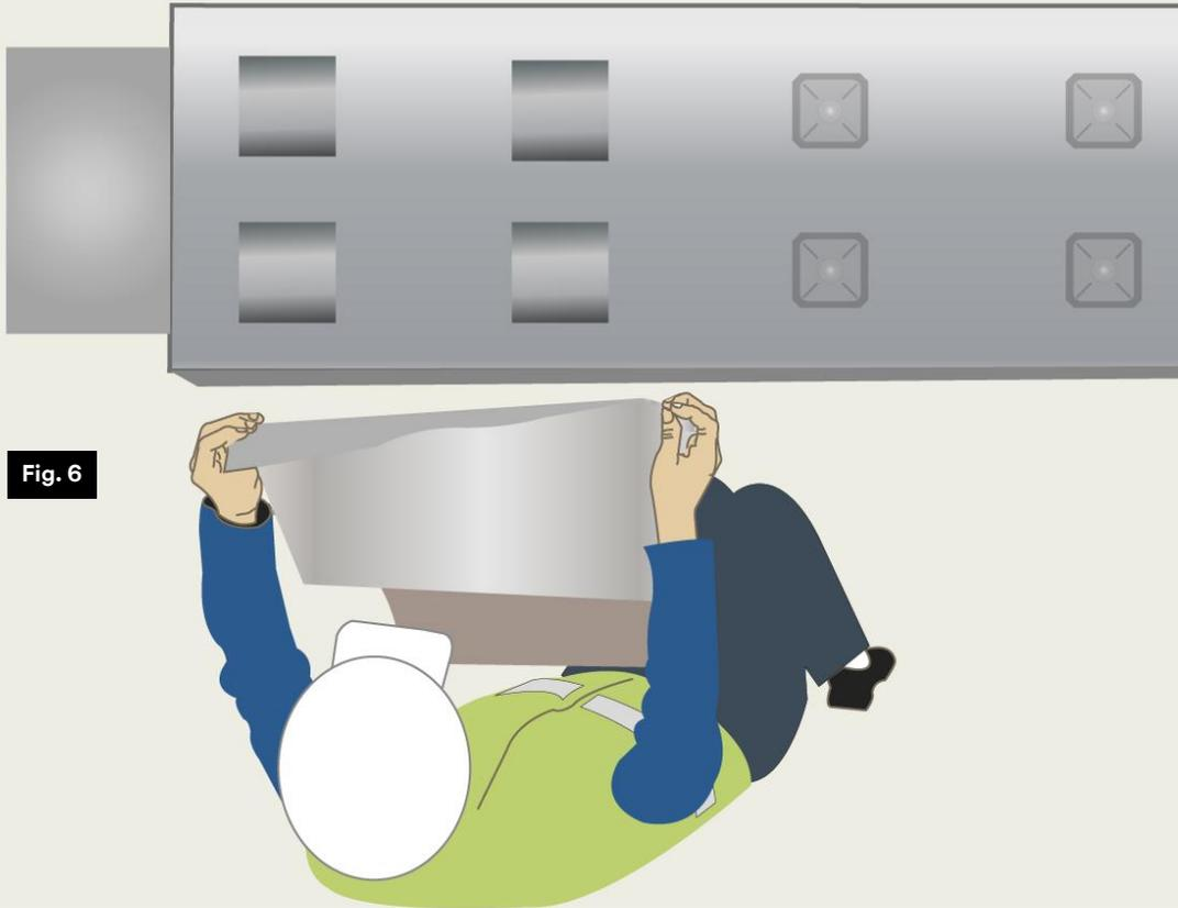
*Figure 6 shows the installer working underneath the insulated duct. He will apply this first sheet of 3M™ VentureClad™ (piece 1) to the insulated duct bottom (where the speed washers have already been covered with 3M™ Venture Tape™).*
