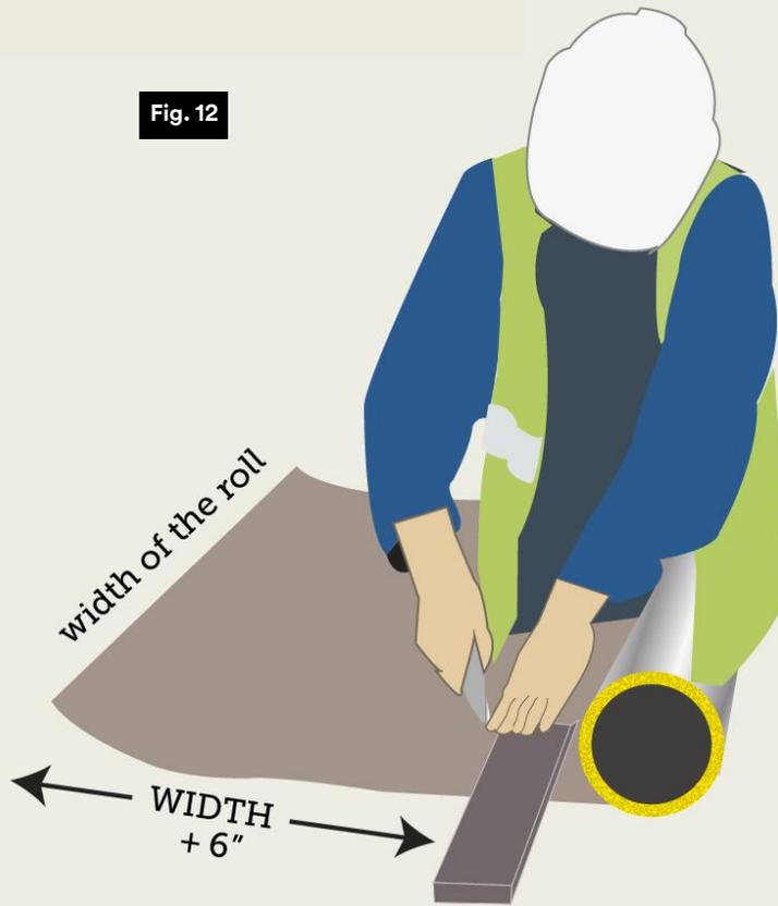
Figure 12 shows the installer cutting a sheet of 3M™ VentureClad™ for the top of the insulated duct (piece 4).
