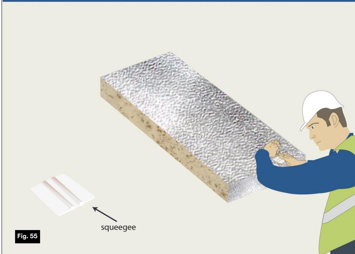
*Figure 55: 3M recommends the installer use a squeegee, as shown above, to make certain that the 3M™ VentureClad™ is well adhered over the entire insulation board surface.*
