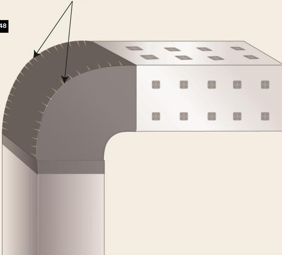
*Figure 48 shows the location for applying the cut Section 4 3M™ VentureClad™ to the elbow heel. Note that it will cover the “feathers” from Sections 1 and 2 after it is applied.*
