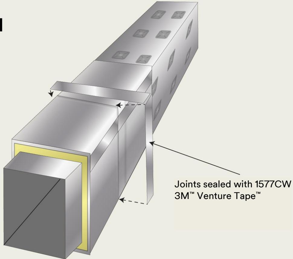
*Figure 19b shows the first step in the addition of 4 inch (100mm) wide 1577CW 3M™ Venture Tape™ over a circumferential 1579GCW 3M™ VentureClad™ butt joint. When using the lighter weight 1577CW 3M™ VentureClad™ jacket, the addition of the tape is unnecessary. Note that the more flexible 1578CW 3M™ Venture Tape™ may also be used to seal the 3M™ VentureClad™ seams.*
