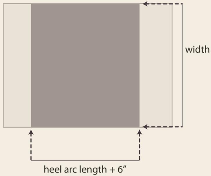
Figure 50 shows the rectangular heel Section 4 to be cut from the 3M™ VentureClad™.
