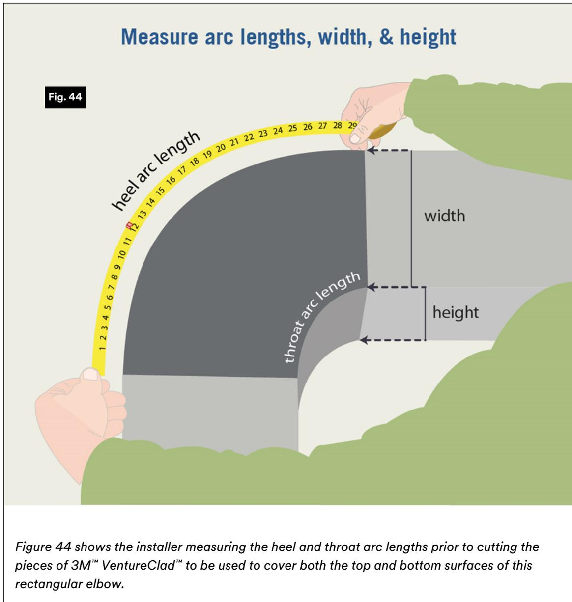
Cut two pieces of 3M™ VentureClad™ as shown below to fit sections 1 and 2 cut feathers in the heel and arc sides.
