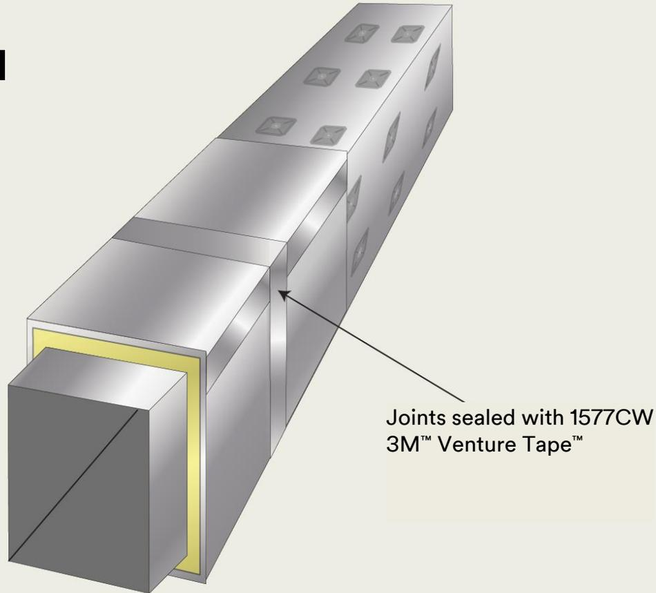
*Figure 19c shows the finished lap and butt joints where the first and second jacket sections join when using 1579GCW 3M™ VentureClad™ as the jacket. Note that they are taped with 4 inch (100mm) wide 1577CW 3M™ Venture Tape™. When using the lighter weight 1577CW 3M™ VentureClad™ as the jacket, taping of the joints like this is unnecessary. Note that the more flexible 1578CW 3M™ Venture Tape™ may also be used to seal the 3M™ VentureClad™ seams.*
