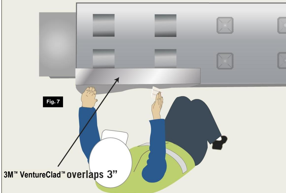
*Figure 7 shows the installer using a squeegee to press the entire surface of the installed 3M™ VentureClad™ piece 1, on the bottom surface of the insulated duct, to assure that there is good adhesion of the 3M™ VentureClad™ jacket to the insulation.*
