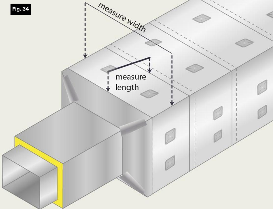
Figure 34 shows measurements to be made for the 3M™ VentureClad™ pieces to be applied to the bottom and top of the larger insulated rectangular duct section that connects to the reducer. Note that prior to applying the 3M™ VentureClad™, each washer should be first covered with a piece of 3M™ Venture Tape™, as shown in Figure 2.
