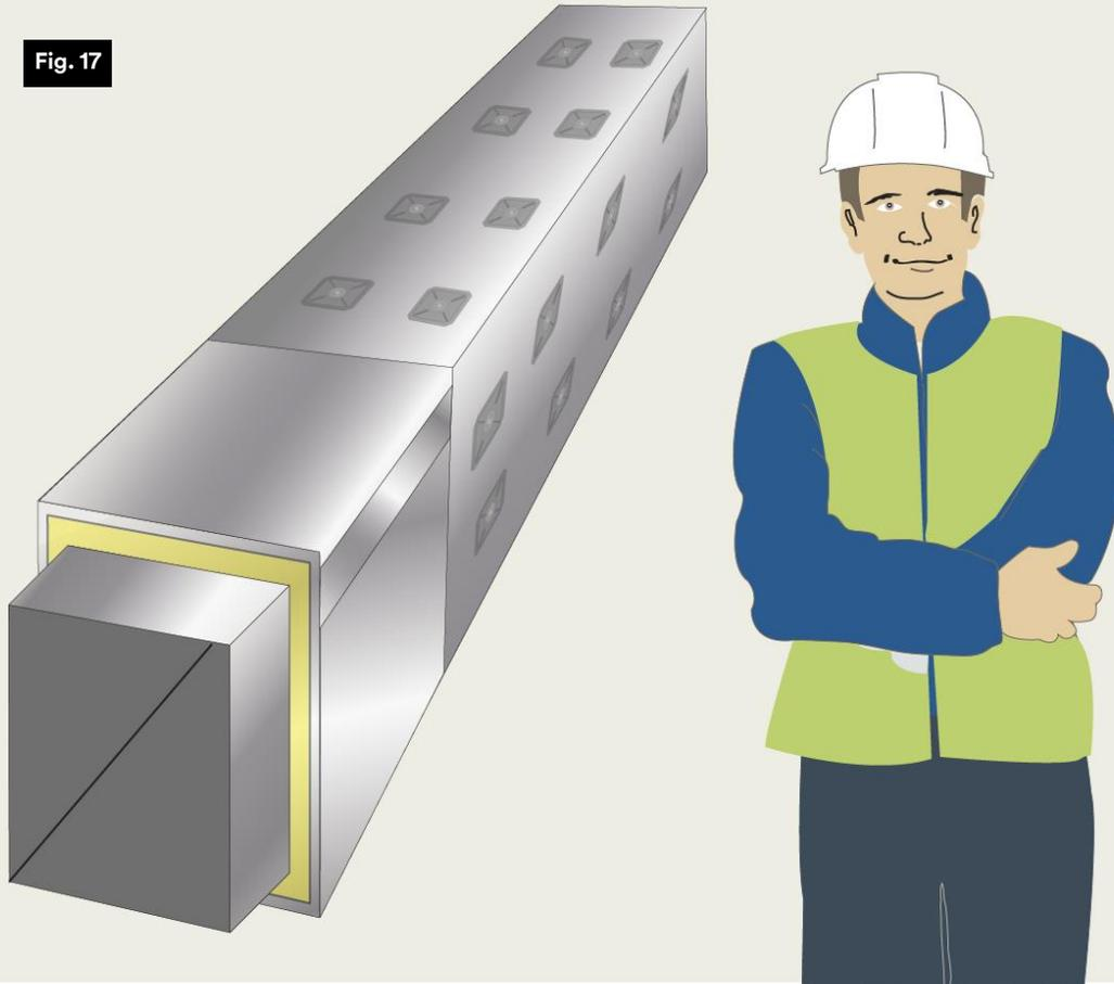
*Figure 17 shows a first section of 3M™ VentureClad™ applied to the insulated duct. Note the joint reinforced with 1577CW 3M™ Venture Tape™ is only necessary when using 1579GCW 3M™ VentureClad™. The next step will be to duplicate this process on the duct section adjacent to this section. Note that the more flexible 1578CW 3M™ Venture Tape™ may also be used to seal the 3M™ VentureClad™ seams.*
