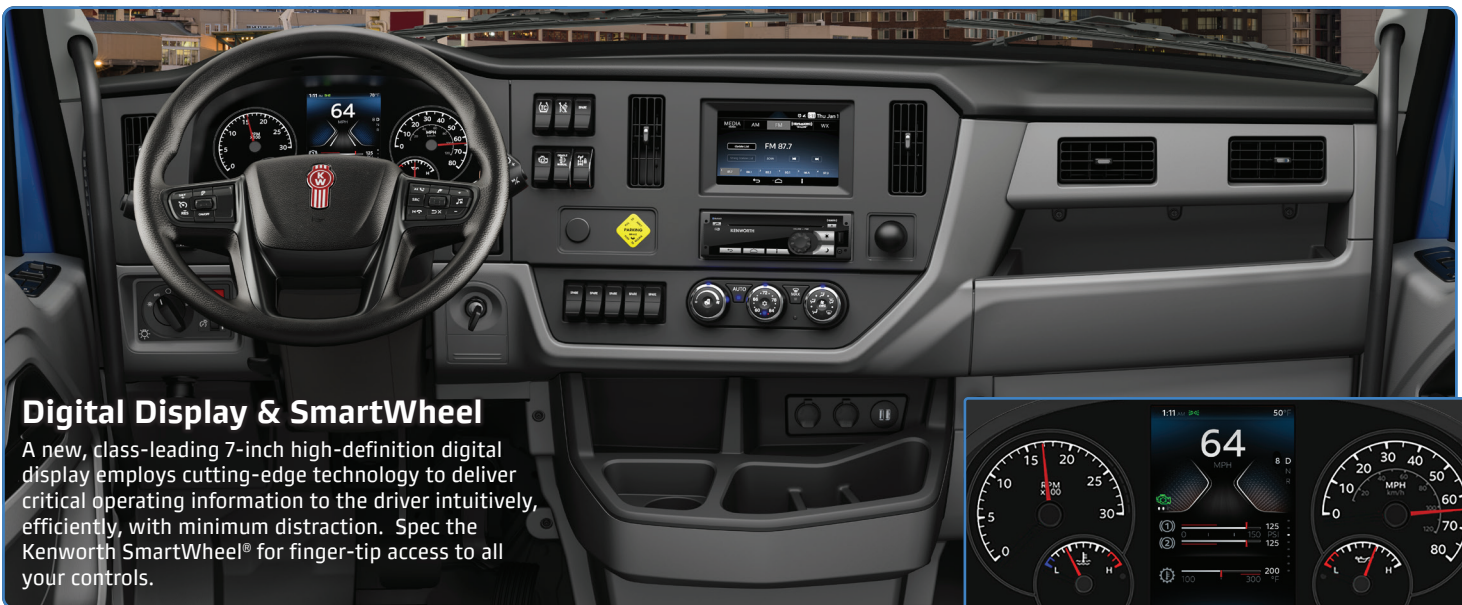
Standard Instrument Panel with 7 Inch Digital Display
