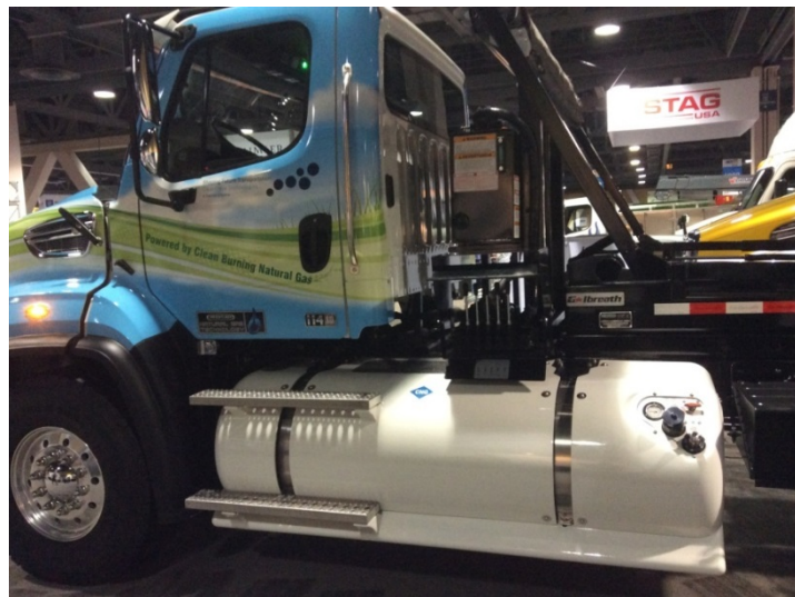
FIGURE 5.1 A 40 DGE COMPRESSED NATURAL GAS TANK INSTALLATION ON A DAY CAB TRACTOR
