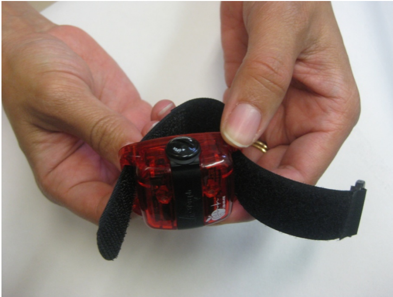
Exhibit 3-11. Threading the wrist strap through the PAM
