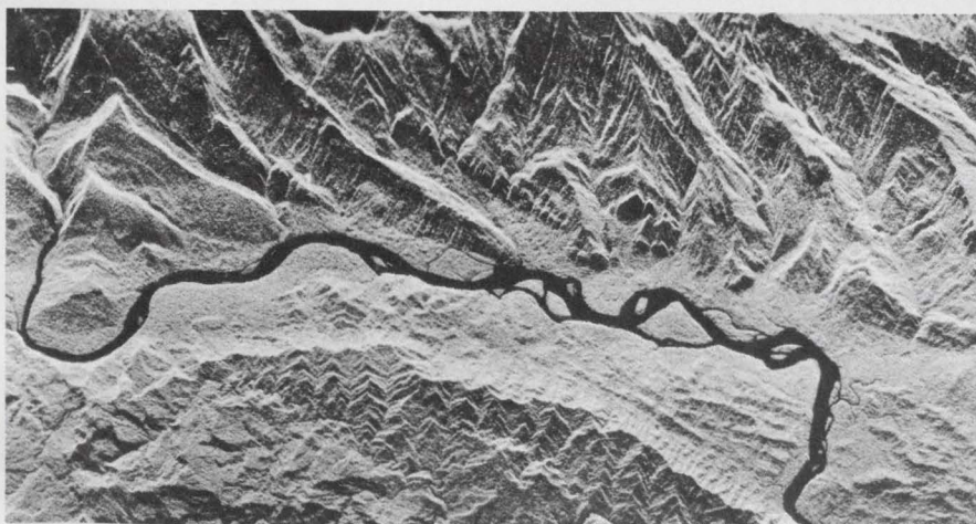
Side look radar image of region of New Guinea resembles aerial photo. Radar is aiding geologists in the search for ore and oil.
