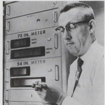
Ultrasonic transducers, held by S. G. Fisher, manager of sonar and flowmeter programs for Westinghouse, will measure waste-water flow in Washington, D. C.
