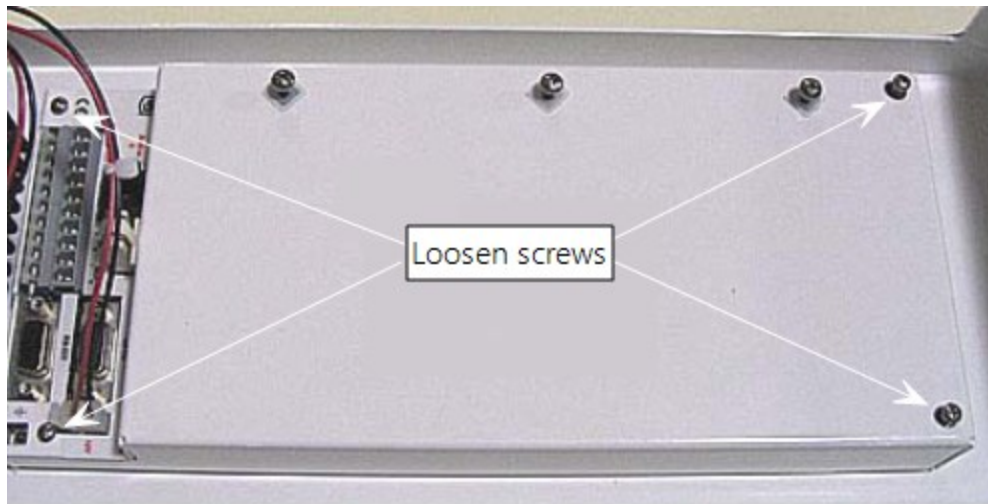
FIGURE 6-13. Screws that secure the electronics cover
