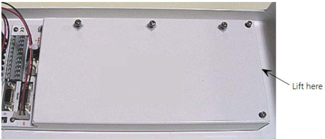
FIGURE 6-14. Removal of the electronics cover
