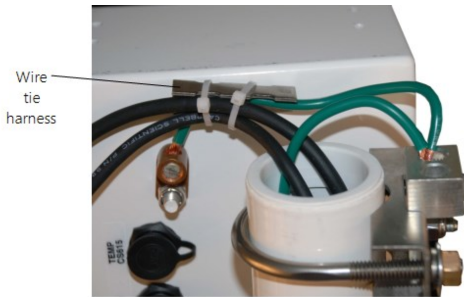
FIGURE 6-44. Cabling strapped to wire tie harness
