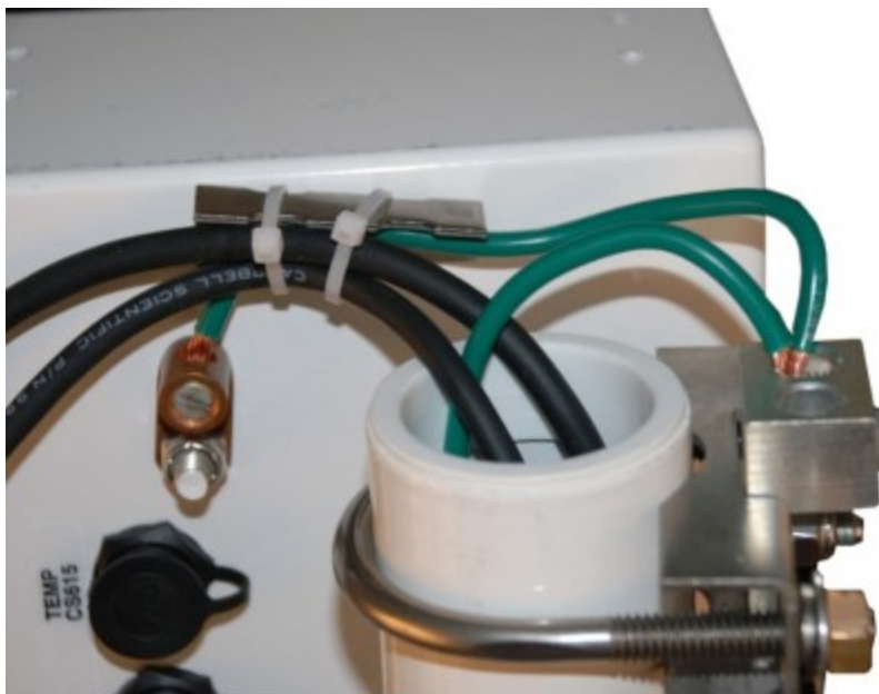
FIGURE 6-39. Grounding to lightning rod clamp
