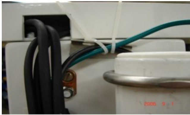
FIGURE 6-28. Loosely wire tie antenna cable
