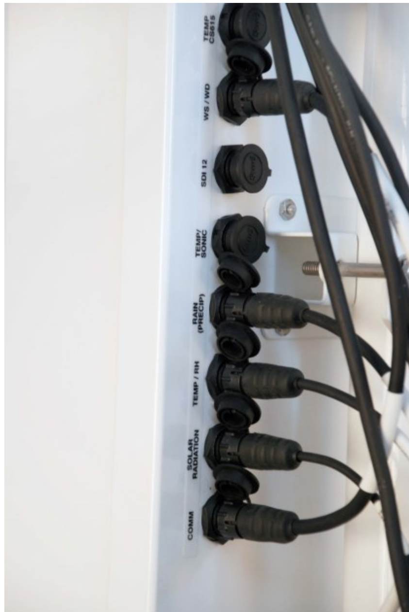
FIGURE 6-21. Connecting sensor cabling to enclosure
