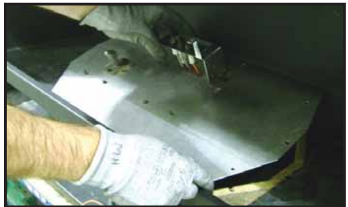
Figure 11.3. Remove Valve Plate
