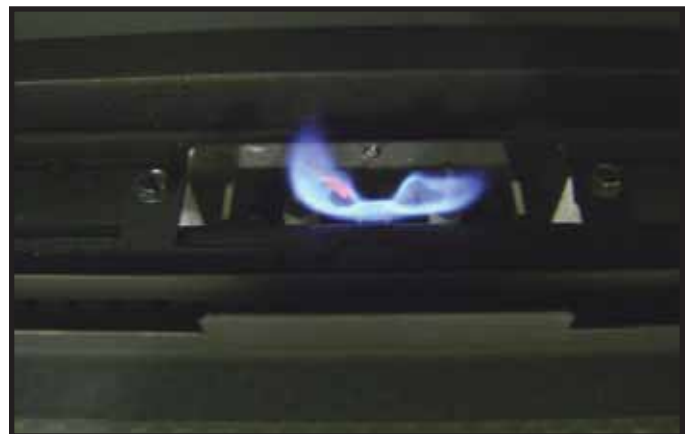
Figure 3.1 IPI Pilot Flame Pattern
