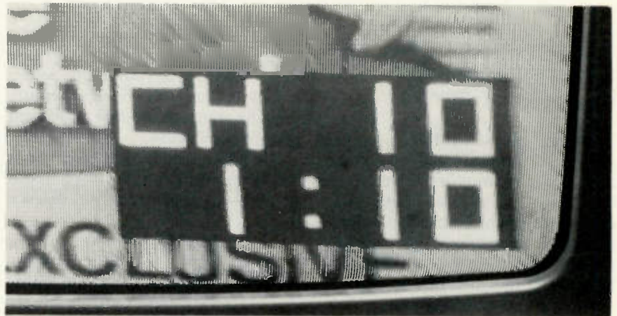
Figure 2 The channel in use and the digital time can be displayed on the TV screen. The channel/time readout has a black background for good visibility. The digits are white but tinted by whatever color is in that area.
