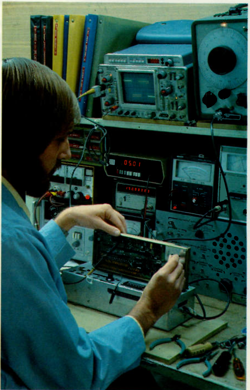
Synthesizer module is tested by a Wulfsberg technician.
